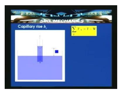
So to that height it will raise then it will stop at that particular portion. That is  $h_c$  which we are going to obtain from the direction. So that is what sigma  $f_v$  is equal to zero yields f = w condition.
