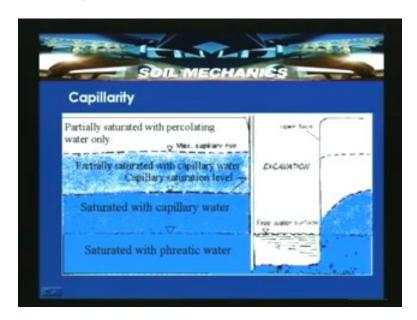
So partially saturated with capillary water that is, this particular one is called a partially saturated with capillary water. Then above that is the percolating water which is nothing but contact water and (Refer Slide Time: 13:37) this is partially saturated capillary zone and this is completely saturated capillary zone and this is our conventional saturated zone which is below the ground water table.
