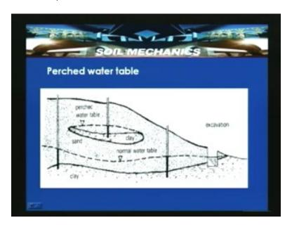
So that is what shown in the above slide, a perched water table condition. This is the normal water table but this could be the localized condition where the water is under perched water conditions, so it is called perched water table.
