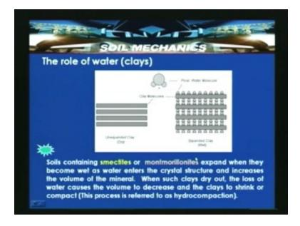
So when such clays dry out, the loss of water causes the volume to decrease and the clays to shrink and compact. So this process is referred as hydro compaction. So when such clays dry out, the loss of water causes the volume to decrease and clays to shrink or
