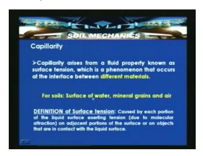
The phenomenon in which water rises above the ground water table against the pull of gravity but is in contact with water table as its source is referred to as capillary rise. The rate of capillary rise is also defined as capillary conductivity. The rate at which this capillarity raise occurs is called capillary conductivity. So water is sucked up in to the pores of the soil mass in this zone on account of the surface tension of water, a manifestation which is referred as a capillary phenomenon.
