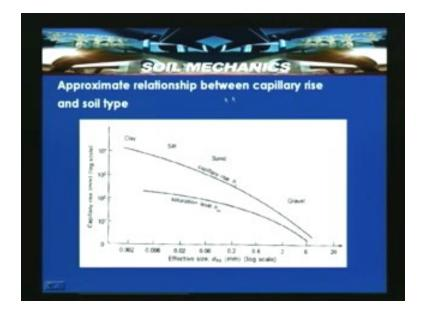
Let us look into the approximate relationship between capillary rise and soil type. The capillary rise is plotted on the log scale on the y-axis and effective size  $d_{10}$  is plotted on the log scale on the x-axis. If you see here this is the capillary rise  $h_c$ , so clay has got around 10,000 mm that is around 10 meters which is followed by silt and then sand
