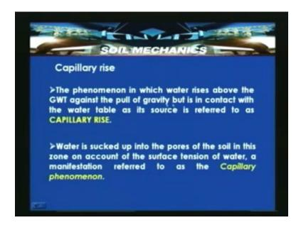
Because of this molecular attraction between materials like inner walls of grains and water and air interface, this water is drawn into the columns of water which are there
