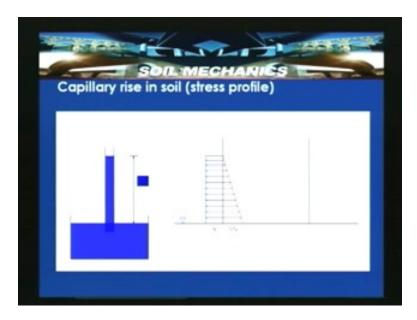
Now this is gamma w  $h_c$ , hydrostatic pressure that is water column which is here exhibits zero pressure here and gamma  $h_c$  here (Refer Slide Time: 43:58). So the net pressure that is the difference of pressure which is indicated in red line to the blue line. That pressure is referred to as the pore water pressure distribution.
