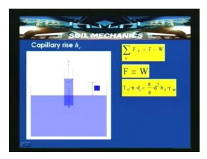
If you write now  $T_0$  .pie .d that is for a chemically clean glass tube alpha =0, then cos alpha =1. So  $T_0$  pie d = pie d square by 4 into  $h_c$  gamma w. This is the self weight of the
