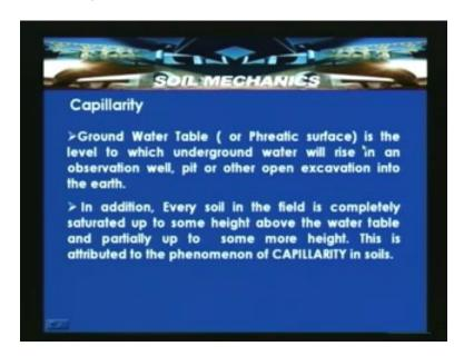
Ground water table or phreatic surface is the level to which the underground water will rise in an observation well, pit or other open excavation into the earth. So in addition every soil in the field is completely saturated up to some height above the water table and partially up to some more height. So we are going to discuss the reasons behind this particular behavior in this class.
