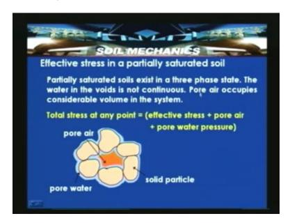
In that situation total stress at any point is equal to effective stress plus pore air pressure plus pore water pressure. In these situations like the total stress at any point is equal to effective stress which is mobilized in the form of an interaction from the grains plus pore air that is when the air is under the pressure, so pore air pressure and pore water pressure.
