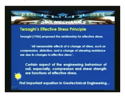
Certain aspect of engineering behavior of soil, especially, compression and shear strength are the functions of effective stress. If there is any change in the effective stress it affects this shear strength characteristic as well as the compression characteristics of a soil. So first important equation in geotechnical engineering. So we have introduced terzaghis effective stress principle. Then we are looking into the much more details about this concept of effective stress.
