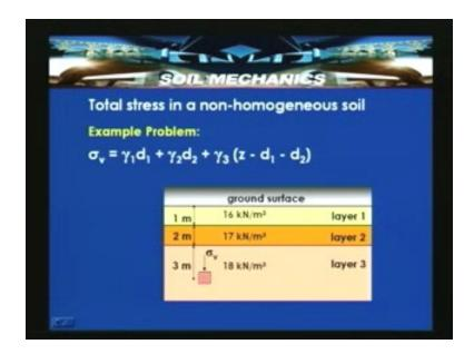
In that case we can determine the resulting vertical stress and it can vary like this. There is a chance of varying slopes because the unit weight is changing with that there is a change in the variation or a slope of this vertical stress with the depth variation. So  $\sigma_v$  is equal to  $104 \text{ kN/} m^2$ , that is what we determined from this example.
