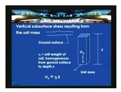
If t is homogeneous then if it is a stratified soil then it is required to be considered depending upon the requirement. This particular vertical subsurface stress is also referred as a geostatic vertical stress. Vertical stress due to strata of different soil types. Suppose if you are having a stratification, like layers which are deposited of thickness z1, z2 and z3 and having unit weights  $\gamma$ 1,  $\gamma$ 2 and  $\gamma$ 3.
