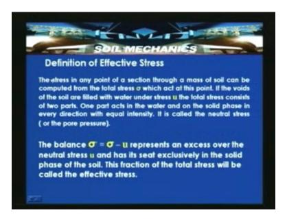
The stress in any point of a section through a mass of soil can be computed from the total stress  $\sigma$  which acts at this point. If the voids of the soil are filled with water under stress u, the total stress consists of 2 parts. One part acts in the water. Previous slide we have seen one part is acting in water and other part is acting in the solid phase in every direction with equal intensity which is called a neutral stress.
