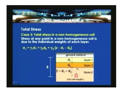
So having seen the cases of homogeneous soil with and without the impounded water. Let us consider a total stress in a non-homogeneous soil which is possible when the stratification takes place during the formation of the soils. When the soil formation takes place, there is a chance of the stratification to occur below the ground surface.
