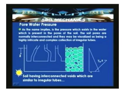
They may be visualized as being a highly intricate and complex collection of irregular tubes. In this particular slide a soil mass, let us assume that this red line which indicates the ground water table and below that all the voids which are filled with water and when this is under no flow conditions, the pressure at the ground water surface which is equivalent to the atmospheric pressure is zero.
