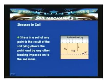
Suppose a loading can be a concentrated load, a line load like a wall which is running over a length l or a line load representing the railway tracks that can be also referred as a line load. It can be a uniformly distributed load representing a fill soil above the certain ground surface. In that case the dotted stress can be due to the self weight as well as due to the vertical stress resulting due to the external loading.
