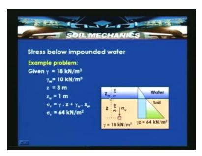
If you look in to it the depths which are given are 3m and 1m. In this example problem we have taken as 1m and unit weight of the soil is  $18 \text{ kN/} m^3$ . As we discussed below it can be soil mass and it can be saturated. In that case if the soil mass is completely saturated like river beds then the  $\gamma$  has to be considered equivalent to  $\gamma$  sat that is the saturated unit weight of the soil mass, while determining the total stress at a particular depth.
