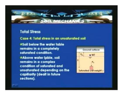
The soil below the water table remains in a completely saturated condition. That is what we discussed in the beginning of this lectures, the soil below the water table remains in a completely saturated condition. Above water table, soil remains in a complex condition of saturated and unsaturated depending on the capillarity which will be dealt in the future lectures.
