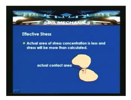
The actual contact area is very less. At the point of contact the stresses are very high, but what we generally determine is that, acting over an imaginary area passing through the grains as well as through the voids can be filled with and without water. For elaborating about this relationship  $\sigma = \sigma' + porewater pressure$ , let us consider a piston analogy.
