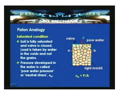
Load is applied through a piston, in that case load is taken by the water in the voids and not the grains. If you assume another analogy, that if I replace this soil skeleton with a spring. In that case what will happen is that the soil skeleton is represented by a spring of certain stiffness and if the same cylinder is filled with water and the valve is closed. When the load is applied and the spring will not experience any compression but the water will be under pressure.
