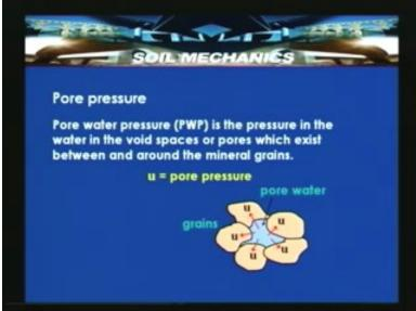
After the introduction of the total stress, it is required for us to understand and define what is meant by a pore water pressure. We have discussed that the void spaces which
