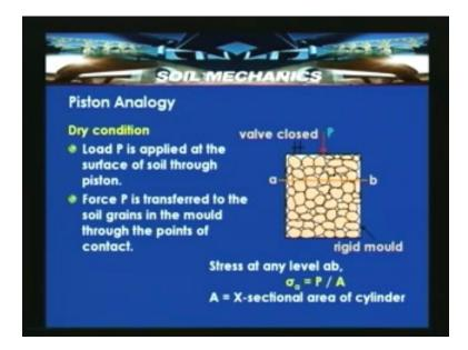
Consider a dry condition assuming that you are having a rigid mould in which the soil grains are filled and p load is applied over a cross sectional area a. So ab is the area which is passing through the voids as well as through the solid grains. And as we have seen the imaginary area passing through the solid grains and as well as the voids are considered in
