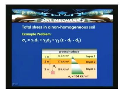
We have seen a homogeneous soil without any impounded water and with impounded water and a stratified soil something like a non-homogeneous soil or stratified soil and then we tried to determine a total stress at a particular depth below the ground surface with these three examples.
