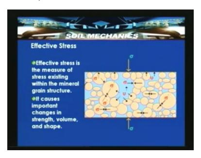
The effective stress is defined as the measure of stress existing within the mineral grain structure. It is shown in the above slide as  $\sigma$ , like a stress which is acting between grain to grain at points of contacts. The u is the pore water pressure existing between the grains and  $\sigma$  is the stress acting at the mineral grain contacts. The  $\sigma$  is the total stress acting over entire soil mass.
