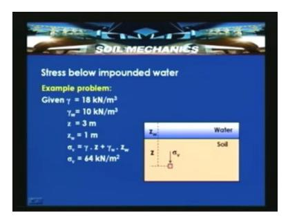
The example problem states like this. Given  $\gamma$  is equal to  $18 \text{kN/} m^3$  and  $\gamma$  w is taken as  $10 \text{ kN/} m^3$ . The z is equal to 3m, zw is equal to 1m,  $\sigma_v$  is equal to  $\gamma$  z +  $\gamma_w$  z, that is
