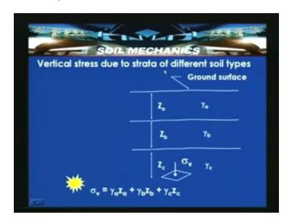
Suppose if you are required to determine stress at a certain depth z below the ground surface, then we have to follow this particular procedure. That means the unit weight which are referred as the layer a  $\gamma_a$ ,  $Z_a$  and  $\gamma_b$ ,  $Z_b$  and  $\gamma_c$ ,  $Z_c$ . The vertical stress  $\sigma_v$
