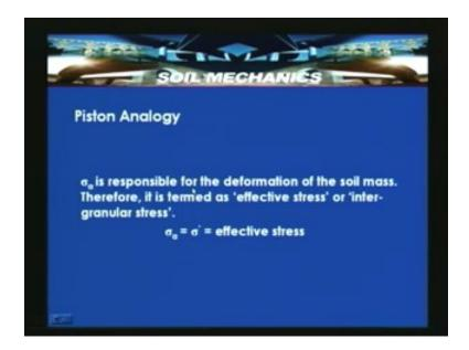
If I look in the piston analogy,  $\sigma_a$  is responsible for the deformation of the soil mass. It is also termed as effective stress. In the case of a dry soil, when there is no water within the voids and it can be referred as  $u_w = 0$ , then whatever the total stress applied is the effective stress which is responsible for the deformation of the soil mass. So  $\sigma = \sigma'$ , this is the effective stress in case of a dry soil mass.
