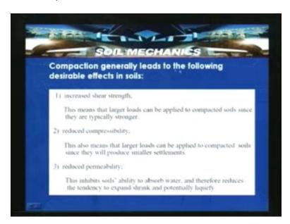
Finally let us look the compaction generally leads to the following desirable effects in field. Our aim is to produce the soil deposit with increased shear strength so that we will
