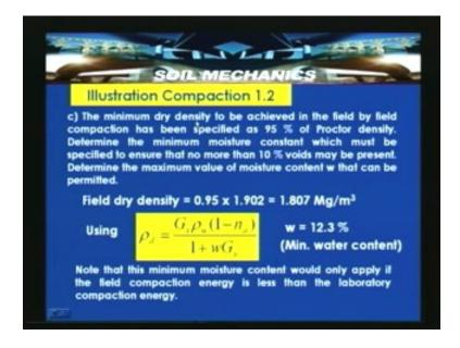
Using  $\rho_{d=} \frac{G_s \rho_w (1-n_a)}{1+wG_s}$  we can determine w=12.3% that is the minimum water content
