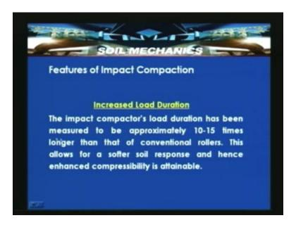
We will now look at the features of the impact compaction which is increased load duration. The impact compactors load duration has been measured to be 10 to 15 times longer than that of conventional rollers. That is one of the important features which are available with the impact compactors. This allows for a softer soil response and hence enhanced compressibility is attainable.
