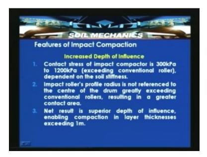
The net result is superior depth of influence, enabling compaction in layer thicknesses exceeding 1m. With these sometimes the large lifts like 1m also can be compacted efficiently with higher dry densities. In the slide below a typical static roller, vibrating roller and an impact roller has been compared.
