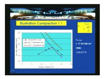
So with these results the maximum dry density at Optimum moisture content of around 15.7% is 17.45kN/ $m^3$ . We can see with the increase in water content there is a maximum dry density or dry unit weight has been reached. Then at a unique water content for that particular type of soil where the optimum moisture content in this case is around 15.17% and then with the increase in the water content beyond the optimum we can see there is a decrease in the dry unit weight.
