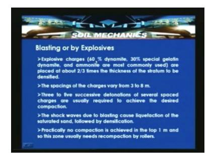
The explosive charges 60% dynamite, 30% special gelatin dynamite and ammonite are most commonly used, are placed about  $\frac{2}{3}$  times the thickness of the stratum to be densified. The spacings of the charges vary from 3 to 8 m. The 3 to 5 successive detonations of several spaced charges are usually required to achieve the desired compaction. A grid of this detonation has to be planned to achieve this degree of compaction.
