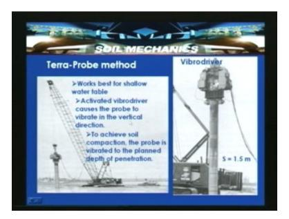
This is a terra-probe method and here it has got a vibrodriver sitting on the probe. It works best for the shallow water table. Suppose the water table is at shallow level that is up to 2 to 3 meters below the ground surface, then this method will be very effective. This method requires densification at spacing which ranging from 1.5 to 2 meters. You can see that s = 1.5 m which is a general thing.
