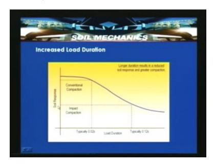
Another feature of the impact compaction is high operating speeds. Landpac impact compactor is the type of compactors which are used generally in the field. It operates at a speed up to 5 times faster and 10 times greater volume per day than the conventional compaction equipment.
