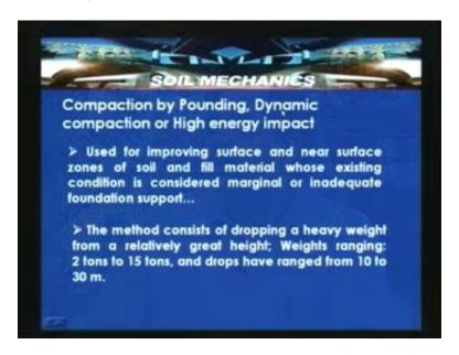
The compaction by pounding, dynamic compaction or high energy impact are used for improving surface and near surface zones of soil and fill material whose existing condition is considered marginal or inadequate foundation support. This method consists of dropping of a heavy weight sometimes ranging from 2 tons to 15 tons at height equivalent to around 10 to 30 m.
