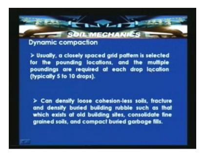
This can densify loose cohesion-less soils, fracture and densify buried building rubble or building depry which exist at the old building sites, consolidate the fine grained soil by dynamic compaction process and compact buried garbage fills. This is widely used in compacting the municipal solid waste fills. That is in the land fill sites the dynamic compaction method is widely used.
