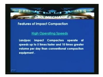
We are trying to compare with the conventional equipment. It says that 5 times faster and 10 times greater volume because larger lift can be compacted, so the volumes of the compaction will be high. Thus we have seen some problems and the solutions for how to
