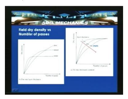
In this slide if you see for a wetter soil the dry density achieved is very much uniform with increasing number of passes. The increasing number of passes on the wetter soil turns out to be futile because it will not have any effect in increasing the dry density. The dryer soil or some natural soil has got the effect which is shown in the first figure. The figure is drawn with dry density versus number of passes for one layer thickness.
