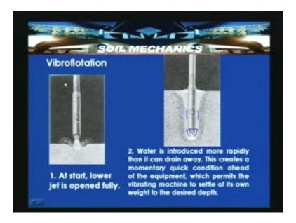
This is the process which is described in the above slide. The 1<sup>st</sup> picture is the vibroflot device in which the bottom jet will open and at the start lower jet is open fully. When it penetrates in to the ground it has to create a quick sand condition where momentarily the soil loses the strength. For that the rate of flow of water should be more than the water draining rate. If I am able to do that then momentarily a quick sand condition can be achieved.
