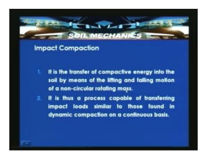
Let us look into another type of compaction method called impact compaction. It is the transfer of compactive active energy into the soil by means of the lifting and falling motion of a non-circular rotating mass. It is thus a process capable of transferring impact loads similar to those found in dynamic compaction on a continuous basis.
