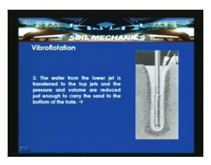
You can see from the slide that the sand is being added. The water from the lower jet is transferred to the top jets. The pressure and volume are reduced just enough to carry the sand to the bottom of the hole. Once the sand supply is started, the bottom is switched off and the water is now opened from the top and sides. You can see the densified soil in the region around the vibroflot.
