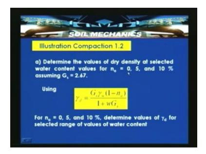
The problem statement is as follows. Part a is n 4 parts. We were asked to determine the values of dry density at selected water content values, ranging from  $n_a$  = 0, 5 and 10% and assuming the specific gravity of the solids as 2.67. Again using  $\gamma_d$ , dry unit weight is equal to a relationship for a partially saturated solid that is  $\gamma_d = \frac{G_{\rm S} \gamma_{\rm w} (1-n_a)}{1+wG_{\rm S}}$ .
