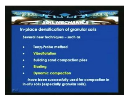
Mostly for loose sandy soils one of the alternatives is to replace some of the loose soils with a column of soil having high relative density. That is when a column of soils which is replaced with high relative density is called a sand compaction pile. This is one method which we can increase the overall load carrying capacity of a soil deposit.
