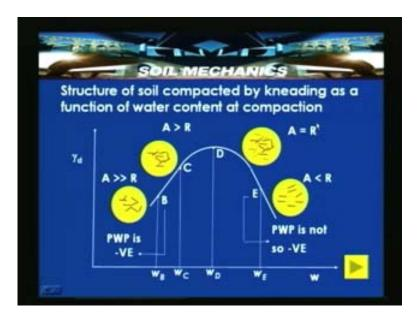
We will try to look into the structure of the soil compacted by kneading as a function of water content at compaction. So, if you look into the reason for an inverted V shaped curve, we said that the reason for an inverted V shape curve for fine-grained soils can be explained in terms of soil structure by T.W. Lambe (1958). The reason for inverted V
