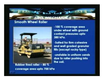
Conventional smooth wheel rollers have 18 tons. Tandem rollers are 1 to 14 tons. Three axle tandem rollers have 12 to 18 tons. This is the conventional weight. The weight can be increased by ballasting the rollers with water or by a heavy sliding weight. So by ballasting with water or by with sand, the weight can be increased. The performance is affected by the load per inch width under the compaction rolls, and the width and the diameter of the rolls. This is about the smooth wheel rollers.
