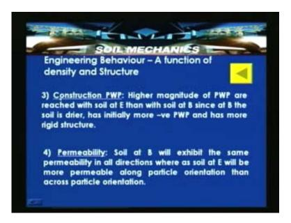
Let us try to look at this. Let us assume that an open arrangement like a truss-like arrangement which is shown here. Then soil at point B with flocculated structure and soil at point E with dispersed structure. Now we are seeing permeability, soil at B will exhibit the same permeability in all directions. Suppose, if I put this as X and Y, then the soil at the point B has got identical permeability in both X and Y directions.
