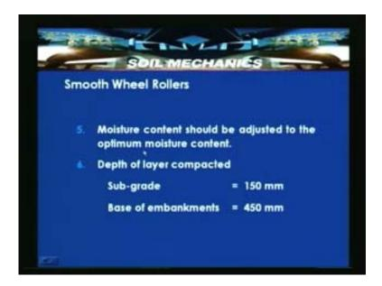
So this is about the smooth wheel rollers. There are also other type of rollers like pneumatic type rollers and sheep's foot rollers.
