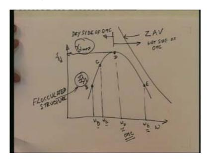
At some limiting stress, what will happen is that this truss-like arrangement collapse and they switch over to a dispersed arrangement. But at very high applied stresses both the soil which is initially flocculated as well as the initially dispersed will have the same structure. So they will exhibit the same compressibility. This is the very important point that should be noted and it will be carried out for understanding the consolidation behavior of soils.
