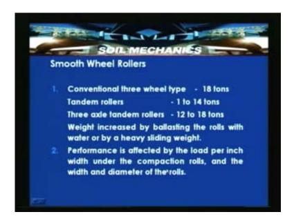
The third point is that load per inch width and diameter control the pressure in the surface layer of soil; dimension of the rolls affect rate with which this pressure decreases with depth. Another point is that suitable for gravels, sands, hardcore, crushed rock and any material where crushing action is needed. So smooth wheel rollers are suitable for gravels, sandy soils, hardcore, crushed rock where some certain extent of crushing is required then this technique will become handy.
