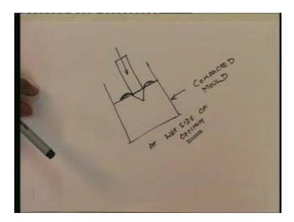
During compaction process these well developed adsorbed water layers surround the clay particles interfere with each other and prevent particles from coming close to each other. This is the case which can happen on the wet side of the optimum. That is why it is very difficult to compact clay soils on the wetter side of the optimum. So this is a typical resulting dispersed structure which is shown here.
