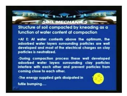
What we have discussed in this particular example is that how the soil structure is transforming as we are proceeding from the left hand side that is on the dry side of the optimum to the wet side of the optimum. Now let us see the influence of the soil structure
