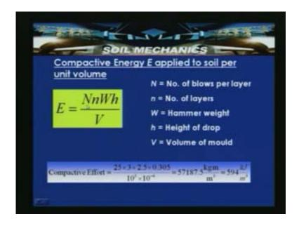
So the standard Proctor test procedure is a continuation if you look into it. The dry density calculations, we knew the volume of the mould and we knew the bulk density of the soil mass at a certain water content that is W by V. So dry density of the soil mass can be calculated by using gamma d is equal to gamma b by 1 plus W the water content.
