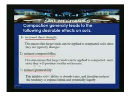
The basic purpose of compacting earth fields such as earth dams and embankments particularly highway embankments and railway embankments and canal is to produce a soil mass that will satisfy two basic criteria; one is the reduction in settlement and increase in shear strength.
