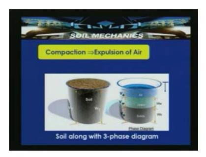
So when loose soils are used for a construction site, compressive mechanical energy is applied to the soil using special equipment to densify the soil or to reduce the void ratio. Densification is nothing but the reduction in the volume of air voids. And this compaction phenomenon is almost an instantaneous phenomenon and soil is always partially saturated and 100% saturation cannot be achieved with the process of compaction.
