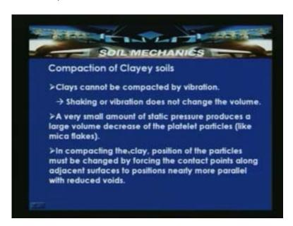
So, if you look particularly into the clay type of soil, the typical particle is of a platelet shape which has got adsorbed water with highly viscous liquid which is surrounding the clay particle and then is also surrounded by free water as shown here. The thickness of the adsorbed free water is depending upon the amount of the available water, this we have discussed in the particle forces lecture. So here in this case like a house of chords loose structure of clay before compaction is shown.
