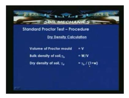
So with this we will be able to establish relationship between water content and dry unit weight or dry density. This particular slide shows a typical moisture content dry unit weight relationship. On the x axis moisture content or water content is plotted and on the y axis dry unit weight or dry density is plotted. So whatever gamma dry or gamma bulk is measured at each of the water content they are plotted here with the points. So by joining the points they form a typical bell shaped curve.
