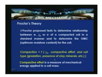
So for measuring the compaction of soils in the laboratory basically the two methods are involved; one is the standard Proctor test, it is named after Proctor 1930 and modified Proctor compaction test which we will be discussing in the next lecture.
