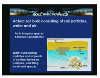
Here, in this slide, the actual soil bulk consisting of the soil particles, water and air is shown. As you can see here, this is the ground surface which is the top surface of the existing ground level in this particular figure. This is the ground water table also called the prioritic surface where the atmospheric pressure is 0, this is the arrangement of the solid grains. The grains which are submerged below the water table are all filled with
