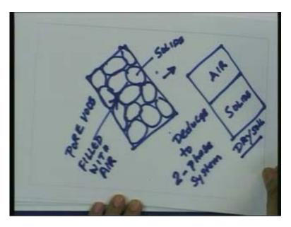
Here, we will see a system with solids and pore voids as idealized. The idealized figure changes like shown which consist of solids and air. These are the soil solids and organic matter. These are pore voids filled with air. So the idealization deduces to a 2-phase
