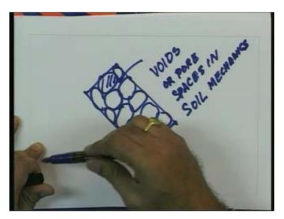
For example, if you look here, the soil mass has got solids which are covered within the soil mass, spaces between these solid particles are called voids or pore spaces in soil mechanics. These are the solid particles and these are the pore spaces. These pore spaces either can be filled with water or air they are usually it is referred like either liquid or gaseous materials.
