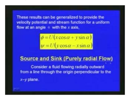
These results can be generalized to provide the velocity potential and stream function for a uniform flow at an angle alpha with the x axis. As shown in the previous slide, these lines are present: phi is equal to Ux and psi is equal to Uy and if you consider certain angle as shown here then we can represent the psi and phi like this. For phi is equal to U into x cos alpha plus y sin alpha and psi is equal to U into y cos alpha minus y x sin alpha
