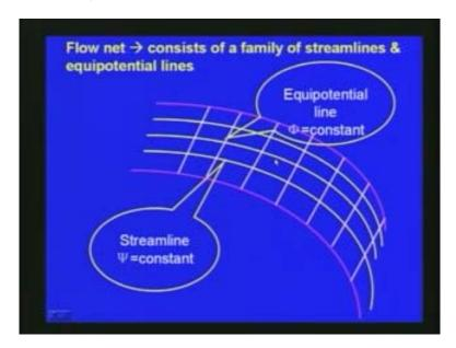
So, here you can see the flow net. Flow net consists of streamlines and equipotential lines; the streamlines are drawn here just like this red color and yellow color and equipotential lines phi is constant is also drawn. So they form the flow net. This flow net concept is very useful in many of the flow net.
