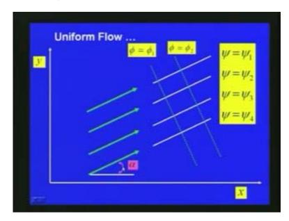
Here also phi<sub>1</sub> and phi<sub>2</sub> represent the equipotential lines and psi<sub>1</sub> psi<sub>2</sub> psi<sub>3</sub> psi<sub>4</sub> represent the streamline.
