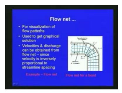
This flow net we can use for visualization of flow patterns as shown here. It can be also used to get graphical solution for fluid flow problems. They can also determine the velocity and discharge can be obtained from the flow net since velocity is inversely proportional to streamline spacing. Here this figure shows a flow net for a fluid flow in a bend so there is a flow through a bend.
