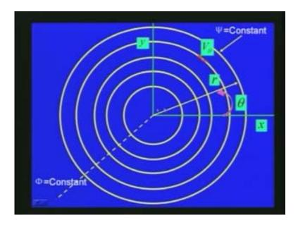
This represents the rotational type which we have discussed here; the velocity, the flow, streamlines are concentric circles and velocity along each streamline is inversely proportional to the distance as shown in this figure. So, phi constant is the dotted lines here and these lines represent the psi constant lines.
