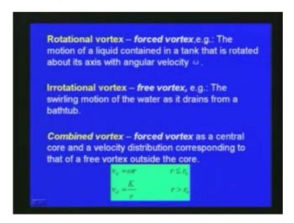
We call the rotational vertex as forced vortex, for example, the motion of a fluid or the motion of a liquid contained in a tank that is rotated about its axis with angular velocity omega. This is called a rotational vortex. Then irrotational vortex, free vortex, for example the swirling motion of the water as it drains from a bathtub. This represents the irrigational vortex.
