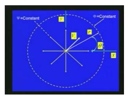
Now, the second kind of the basic or elementary potential flow which we represent is called the source and sinks; the source and sink is purely radial flow type. So the fluid flow is radialy outward from the origin perpendicular to the xy plane only we have to consider the  $y_r$ - the radial velocity here and  $y_r$ - the radial velocity here and  $y_r$ - the phi is equal to constant. This line represents  $y_r$ - the radial velocity here and  $y_r$ - the phi is equal to constant.
