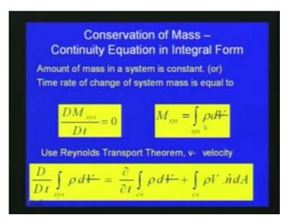
Now, we discuss the conservation of mass, the continuity equation with respect to the integral form of approach. We have seen that just like in fluid mechanics also the fundamental theories are based up on the consideration of mass, consideration of momentum and consideration of energy, so most of the basic principles of basic theories are developed based up on conservation of mass momentum and consideration of energy.
