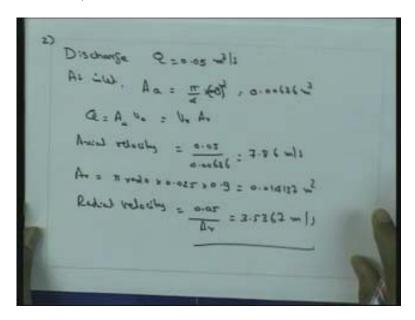
So, the discharge can be written as Q is equal to 0.05 meter cube per second Q is equal to that is discharge is equal to 50 liter per second or it can be written as 0.05 meter cube per second at inlet. So, the inlet is here. At inlet we can write, the discharge is equal to area of cross section multiplied by the axial velocity so that what is entering that should go through impeller.
