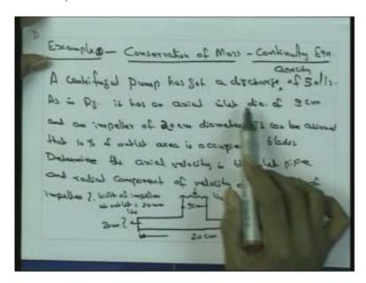
So a problem here is a centrifuged pump has got a discharge capacity of 50 liters per second as shown in figure it has an axial inlet diameter of 9 centimeter and then impeller of 20 centimeter diameter so it can be assume the 10 percent of outlet area is occupied by blades so we have to determine the axial velocity in the inlet pipe and the radio component of velocity like the outer impeller.
