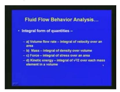
So integral form of quantities we can see that most of the quantities we can described in terms of integral form just like for example the volume flow rate it is the integral of velocity over an areas so if we consider the volume of the discharge passing through integral of velocity over an area that is the discharge for volume of flow rate and second for example the mass if we consider the mass it is the integral of density over volume.
