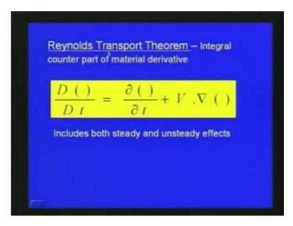
Reynolds transport theorem with respect to the counter part of the material derivative, we can write as D of Dt of the particular parameter which we are dealing equal to del by del t of the parameter plus V dot product del of the parameter, so this include both the steady and unsteady effects we have seen, so this gives the Reynolds transport theorem with respect to the material.
