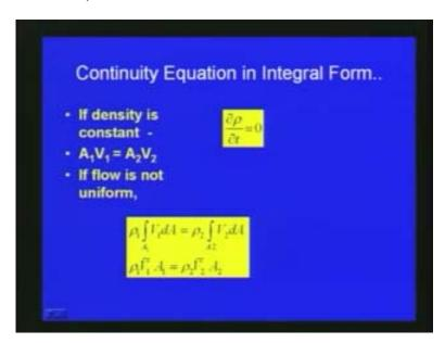
Finally, the continuity equation integral form if the system is at steady state or if there is no change with respect to the density that means there is del rho by del t that means no change of density with respect to time this can be written as 0.
