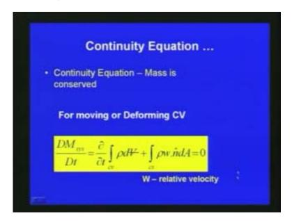
The continuity equation as we have seen here the mass is concerned and we have also seen that there can be or deforming a control volume so in that case the with respect to the continuity equation of the conservation of the mass we can write DM system Dt is equal to del by del t of control volume rho dv plus all the control surface rho w instead of V here we are using rho w n hat dA is equal to 0.
