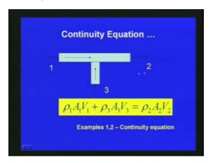
For example, if you consider a pipe with branch like in this slide so here we can express the continuity equation like here. At the section 1 if  $V_1$  is the velocity and area of cross section is  $A_1$  and the density here is  $rho_1$  and at section here at three if the velocity is  $V_3$  and area of cross section is  $A_3$  and density is  $rho_3$  and then here this location the density is  $rho_2$  and  $A_2$  is the area cross section  $V_2$  is the velocity.
