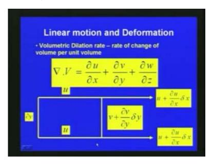
This is the conservation of mass of the continuity equation which is one of the basic equations which is used in all the fluid flow analysis, so this is the integral form. Now we will be discussing about the differential form later. Before going to the differential form of the continuity equation here you can we will see in this slide the linear motion and
