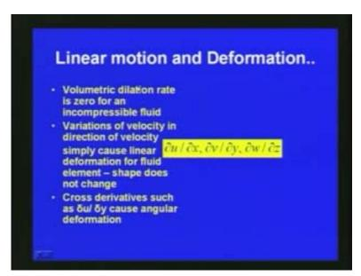
Now, we can see the volumetric dilation rate is 0 for an incompressible fluid, so when we are dealing with incompressible fluid volumetric dilation rate is 0, so we can write the variation of velocity in direction of velocity is del u by del x, del v by del y and del w by del z, since we are dealing the velocity components in xyz direction.
