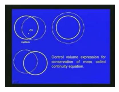
Now, as we can see in this slide the control volume it can here, this is the system which we are considering and the control volume is inside what is there and then what changes taking place with respect to whether with in the control surface that is what we are describing so control volume expression for conservation of mass called the continuity equation.
