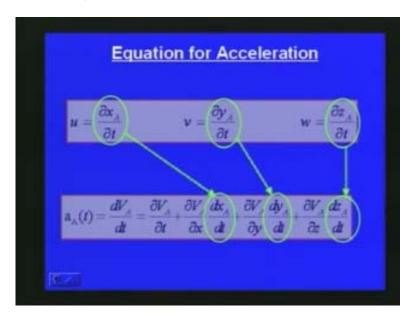
Here this dxa by dt can be represent as u and  $dy_A$  by dt can be represent as v and  $dz_A$  by dt can be represent as w. Finally, if you substitute the total acceleration can be represented as shown in the slide.
