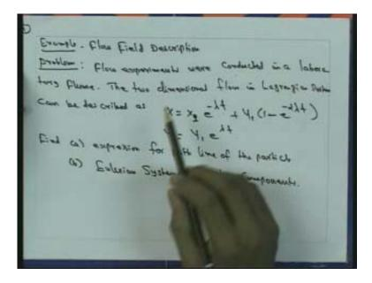
In an experiment of flow description were conducted in laboratory flow, the 2 dimensional flow in a lagrangian system is already obtained as x is equal to  $x_1$  into e to
