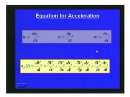
In the legrangian description than we will be writing with respect to u is equal to del  $X_A$  by del t the velocity described as here we will consider the equation for acceleration. The velocity component in x direction u is equal to del  $X_A$  by del t and v is del v by del v as shown in this figure.
