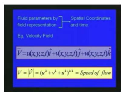
By field representation as I mentioned earlier the fluid moment is then you consider the fluid moment it the moment is in with respect to space as well as time. If you consider the space we consider the 3 dimensional motion of a fluid with respect to xyz axis time t will be all will be there.
