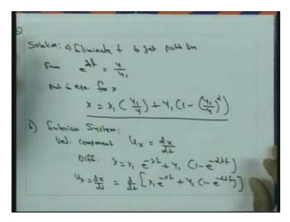
We will eliminate it t the time component to get path line from the second equation from second equation you will get e to the power lambda t is equal to y by  $y_1$  equation is given y is equal to  $y_1$  in e to the power lambda t. The from that we can write e to the power
