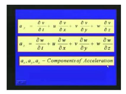
As ay is equal to del v by del t plus u into del v by del x plus v into del v by del y plus w into del v by del z acceleration in z direction can be written as del w by del t plus u del w by del x plus v into del w by del y plus w into del w by del z.
