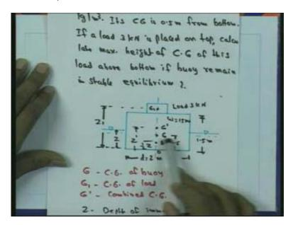
Its center of gravity is point five meter from the bottom if a load 3 Kilo Newton is placed on the top. Calculate the maxim height of the center of gravity of this load above the bottom if buoy remain in stable equilibrium?
