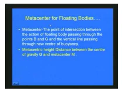
Metacenter we can define as metacenter is the point of intersection between action of floating body passing through the point b the center of buoyancy and g the center of gravity and the vertical line passing through the new center of buoyancy.
