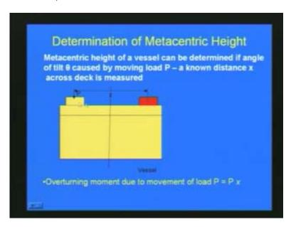
You can see there is a weight put on one side of the vessel and then we are moving this vessel from one position say this is old position of the vessel we are moving this vessel this body on the vessel the small body on the vessel from one position to another so that there will be a small displacement will be taking place and then we what will determine the metacentric height.
