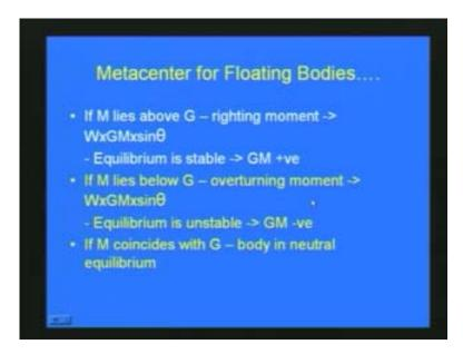
So the metacenter floating bodies it is very important we have to determine the metacenter and we have to see what is the position of the metacenter that we can determine the weather bodies in stable conditions or unstable conditions. Here if m the metacenter lies above g so that righting moment may be w into w the weight of the floating body gm the metacenter height into sin theta.
