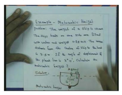
There is a floating body like this and there is a small weight is placed like here. So we want to determine the metacenteric height. So the problem is the weight of the ship is 150 Newton the ship boats or one side are filled with water and weight 0.85 atoms Newton. The mean distance from the center of ship to the boat is 8.5 meter that means this
