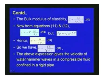
Now let us introduce this with respect to the fluid movement, let us introduce this Bulk modulus of elasticity of the system. If you write the Bulk modulus of elasticity K is equal to minus delta p by delta rho by  $rho_0$  as in equation number 12.
