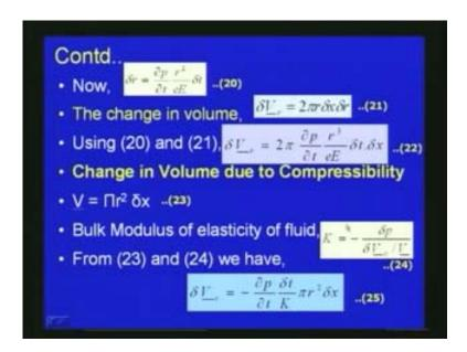
Now we can write delta r is equal to del p by del t into r square by e into capital E which is the Young modulus into delta t as in equation number 20.
