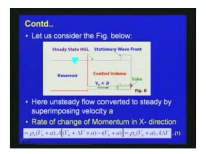
Now here say if we consider the same systems as we discussed, so here now the velocity here is  $V_0$  plus a and then here at the velocity changes. Here, the unsteady flow, as I mentioned is converted to steady state by superimposing the velocity 'a'. So here, that is what we are done. Now we can find out what is the rate of change of momentum. Here we can see that with respect to the change in velocity there will be rate a change of momentum.
