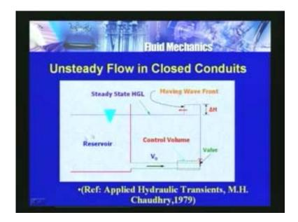
If we consider simple system like this here, there is a reservoir and then the reservoir pipe is connected or a conduit is connected like this and then to develop the theories with respect to such a system - a simplified system - say we assume here there is a valve and then due to sudden showdown of the valve, what happens with respect to the water hammer or hydraulic transients.
