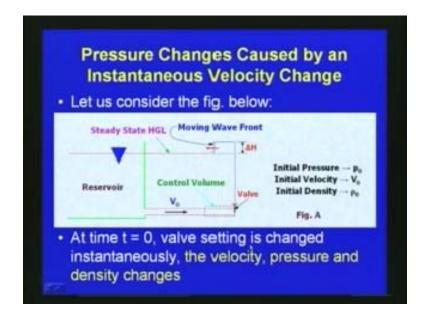
Now, we want to find out some relationship to connect with respect to the water hammer the velocity of the wave front and then how this can be connected with respect to the pressure which is building up, with respect to the sudden valve closure - so that is what we want to find out.
