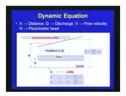
To derive this dynamic equation and continuity equation we consider here say there is the flow through a pipe here over the close conduit and flow is going this direction. Here the radius of the pipe is r and here is datum and here the total head is the piezometric head here H and the here it is plotted the instantaneous hydraulic gradient line is plotted for the system. Here we consider two sections: at section all here at distance x from the origin.
