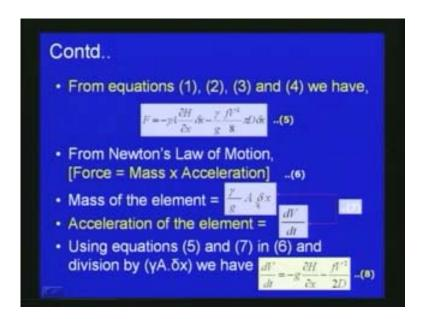
So from equations 1, 2, 3, and 4 we can write F is equal to minus gamma A del h by del x into delta x minus gamma g into fV squared by 8 into pi D into delta x.
