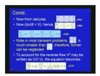
So now from calculus we can write this dv by dt, which is acceleration is equal to del V by del t plus del V by del x into dx by dt, since dx by dt is equal to velocity V, we can write dv by dt is equal to del v by del t plus v into del v by del x as in equation number 9 b. So that finally we can write the dynamic equation as del V by del t plus V into del V by del x plus g into del H by del x plus fV square by 2D is equal to 0, as in equation number 10.
