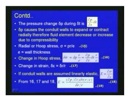
Then the pressure change delta p during delta t the time, change in time we can write as del p by del t into delta t. So the delta p causes the conduit walls to expand or contract radially. Therefore, the fluid element decrease or increase due to the compressibility effect.
