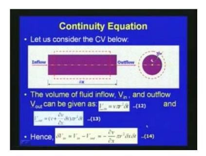
This is the dynamic equation which we have derived based upon the Newton second law. Now the second equation for the unsteady flow through closed conduits or pipe we can obtain from the continuity equation; so to derive the continuity equation let as consider a system like this.
