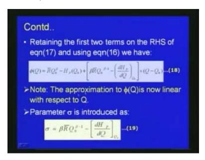
We are using the Taylor series by retaining the first two terms of the right hand side equation 17 and using equation 16. We can show phi Q equal to R bar  $Q_0$  power beta minus  $H_p$   $Q_0$  plus beta R bar  $Q_0$  to the power beta minus 1 minus d  $H_p$  by d Q whole into Q minus  $Q_0$  as given in equation number 18. Here, this approximation of to phi Q is now linear Q.
