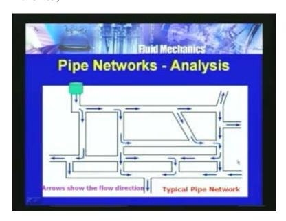
The pipe network, we have seen that, it will number of loops. Most of the time, we have to assume the flow direction and flow through each pipe, we have seen this aspect.
