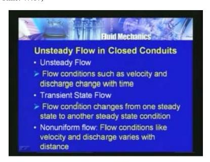
The unsteady flow as we may have discussed earlier, flow conditions such as; velocity and discharges change time. Sometimes this flow is set to be transient state flow.
