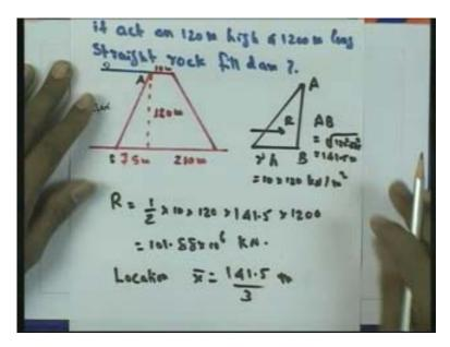
Will be r is equal to half into this base gamma into h in this length AB this height AB which we are considering in this inclined height. So that will be 141.05 which we have already determined multiplied by the width of the length of the dam that is 1200 meters.
