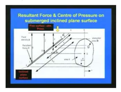
In today's lecture, we will discuss the resultant force and center of pressure on submerge inclined surface, inclined plane surface.
