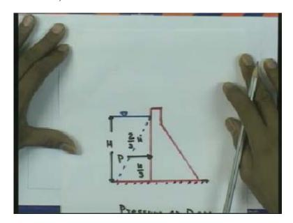
Here, you can see if it concrete dam here, so if you want to find out the certain force and center of pressure so here, this gamma h below on this surface is the pressure here, and then total pressure is the area of this triangle. So that is equal to gamma A xbar in this case we can see the gamma h into h by 2 is the per unit and you can multiplied by the width of the where the dam is river width or where that section is there.
