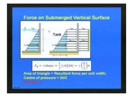
Now, we will discuss. So vertical surface instead of inclined plane if you consider the vertical surface as you can see here in this slide. Put the case of vertical surface this is a time, where we want to find what will be the resultant force acting on this particular whole here. So here you can see this height, the height of the liquid of the water here is h and here this surface of the time is affected by the atmospheric pressure.
