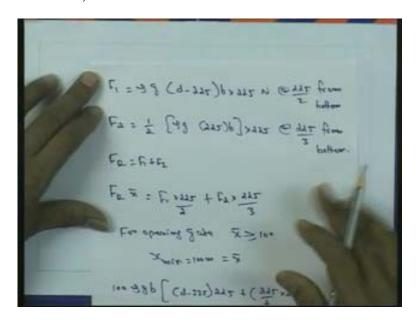
So that is  $F_1$  is equal to rho into g into d minus 225 into b into 225 Newton acting as 225 by 2 from the bottom. So that is correspond to, this force distribution  $F_1$  and then we can determine  $F_2$  for this triangular pressure distribution is concerned  $F_2$  is equal to half into rho into g into 225 into b multiplied by 225 that will be acting this 225 by 3 from bottom.
