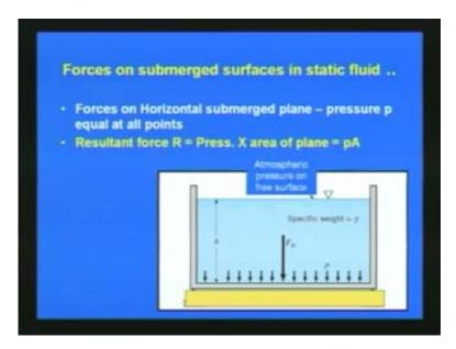
Also we have seen the forces on submerged surfaces in static fluid and the resultant forces pressure into area of plane that is equal to P into A as shown in this slide.
