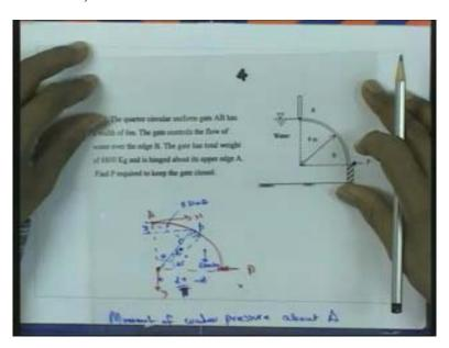
There is a problem statement is the quarter circular uniform gate. There is a gate AB has a width of 6 meter and the gate controls the flow of water over the edge B the gate has total weight of 6800 kilo gram and its hinged about it upper edge A, find P the force
