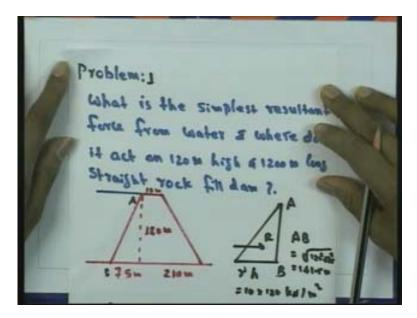
The problem here, we are discussing is, there is rock fill dam like this, so we want to determine the what is the simplest resultant force from water and where does it act on? 120 meter height and twelve hundred meter long, straight rock fill dam that is the problem.
