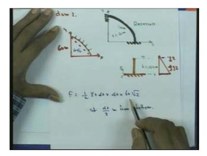
Which this case is acting? So the total the simplest resultant which in this case for this arch dam will be 1 by 2 gamma 40 into 40 into 60 root 2. Where gamma is the specific weight of water and this will be acting at 40 by 3 from the bottom. So this is the case how to find out this simplest resultant force of the hydrostatic pressure in an arch dam. So one more problem we will consider so here the last problem here.
