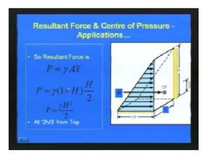
Here, P is equal to gamma H square by 2 for unit to, so then it is acting 2h by 3 from the top and h by 3 from the bottom, so this also we have seen.
