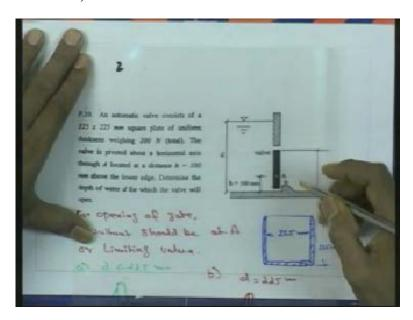
There is a valve here which at this point and below the downstream this [] the water depth is 225 millimeter and then this; the gate is the pipe pivoted at h is equal to 100 millimeter like this.
