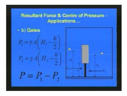
So [] gate are very much used in the case of many of the hydraulic structures as far as canals or dams are concerned. So how we can determine the resultant force?
