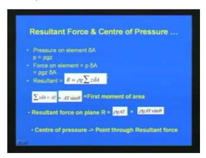
Now, the resultant force and center of pressure, so the pressure on element delta A as we have seen in the previous slide is, P is equal to rho into g into z where, rho is the density of fluid, g is the acceleration due to gravity, and z is the depth at which the element delta A is concerned.
