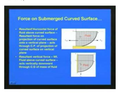
Here, the resultant force the resultant horizontal force of fluid above the curved surface is the resultant force on projection of curved surface. We can project the curved surface to a vertical plane, this and then we can find out, what will be the force acting on those vertical surfaces. So that will give the resultant horizontal force. The case of this curved
