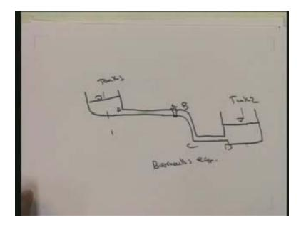
So based upon it when we design a pipe, for example here let us assume a pipe flow system starting from a tank and then it is going to another tank like this for such as system there is valve or a bench and exit lot entrance is like this. So here what generally we can use the Bernoulli's equation to show these kinds of problems. Between two sections assume that when we consider if this is a b c d and then between the tank 1 or server 1 and this is tank 2.
