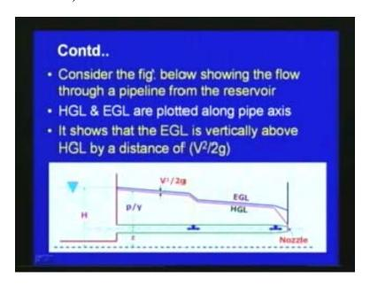
If you consider the figure here, this figure so there is a tank or reservoir higher then the pipe going like this and then it is nozzle here at the end of this pipe. If this is the datum then we can see that data available thrust will datum is h with respect to the reserved wire and then we can find out this p by g and then p g plus z. So this red line here that will be the hydraulic radian line and then if we add the v square by 2g which is the velocity here v square by 2g.
