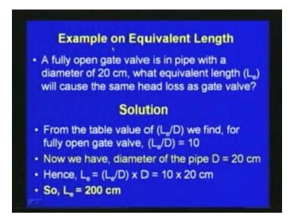
A fully open gate value is in pipe with a diameter 20 centimeter. What equivalent length 1 e will cause the same head loss as gate valve? So now the question here is same we have
