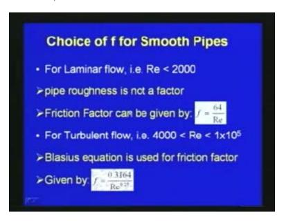
We can directly obtain the pipe reference the friction factor, directly calculate physical to 64 byte Renolds number and for turbulent flow, up to this between four thousands to the into between the range of 10 to the power of 5 to 4 four thousands Renolds number range, blasius calculated this friction factors equal to 0.3164 divide by r e to the power 0.25.
