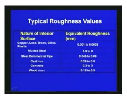
Typical roughness values are given, for example, copper, lead, brass, glass, and plastic. So phis (34:55) of this material and the roughness vary from 0.001 to 0.0025 mm and then if the pipe is riveted steel it goes from large value like 0.929 mm and steel commercial pipe this roughness equivalent roughness varies from 0.045 to 0.09, cast iron pipe is concerned then we can see that increment reference high varies from 0.25 to 0.8 mille meter and concrete pipe depending upon the finishes.
