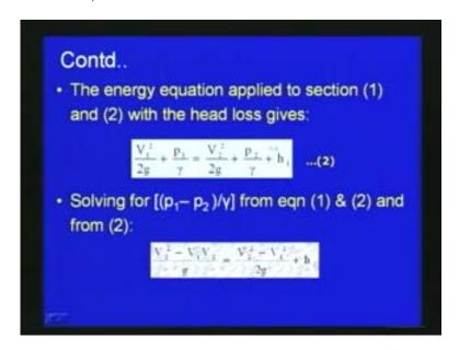
So now solving by  $p_1$  minus  $p_2$  by g from this equation and if we use this equation 1 a and 1 b and we can write v2 square minus  $v_1$   $v_2$  by g is equal to  $v_2$  square minus v1 square by 2 g plus  $h_1$ .
