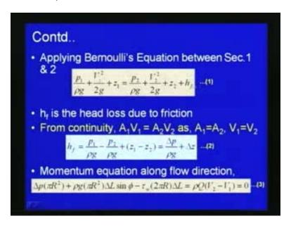
Let it be represented as h f. So, by applying the Bernoulli's equation between section 1 and 2 we can write  $p_1$  by rho g plus  $p_1$  square by 2 g plus  $z_1$  equal to  $p_2$  by rho g plus  $v_2$  square by 2 g plus  $z_2$  plus h f. This is obtained from the Bernoulli's equations. So here h f is the loss with respect to the friction with respect to the viscosity effect between section
