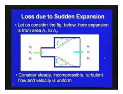
Flow is coming like this and then expanses. Here let as consider 2 sections here section 1 and section 2 and section 1 area flow section is a1 and velocity average velocity  $v_1$  and pressure p1 and section 2 area flow section  $a_2$  and velocity is  $v_2$  and pressure is p2. Let us consider the flow to be steady and fluid incompressible turbulent flow and velocity is uniform with respect to the assumption.
