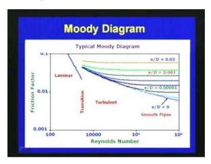
So here this line shows the moody's diagram here the x axes the Renolds number is represented and on this access the friction factor is given and here the curves are given for various e by d ratio where e is the represent height the relative reference e by d is the diameter e by d is equal to 0.03 like that for various values, the roughness for various roughness are e by d issues and the Renolds number the friction factories even here.
