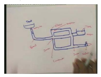
So as we have seen, for example if a connecting here the vary say time here and now if we are connecting, putting a pipe line like this with various branches and then various joints, you can see now in a such a system we may be distributing either for water supply or may be for various other kinds of network.
