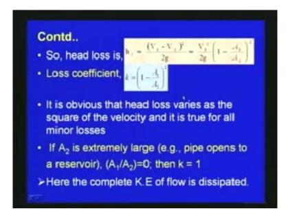
We obtain from equation using equation 1 a and 1 b and equation number 2. So finally we get the head loss h 1 is equal to  $v_1$  minus  $v_2$  whole square by 2 g. That can be
