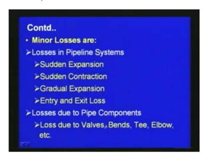
Where v is the average velocity, k is the coefficient for minor loss is the acceleration due to gravity when k is determined experimentally for various fittings and geometric changes of interest in piping system. As we discussed earlier depending upon a problem there would be different kinds of joint are different kinds of contract expansion (42.12) junction etc.
