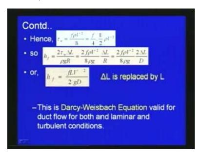
Hence,  $tau_w$  is equal to f rho v square by 8 that can be written as f by 4 into half rho v square. We can write h f is equal to 2 into  $tau_w$  delta l by rho g r. That is equal to up to substituting for  $tau_w$  h<sub>f</sub> is equal to 2 f rho v square and delta l by 8 rho g into r.
