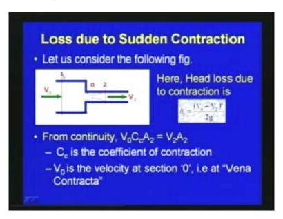
Here this section 1, this is the large diameter then smaller diameter, so here the velocity is v1 at section 1 and here the velocity section 2 is v2 and then we can see that in the case of
