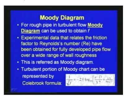
First let us see the moody diagram. This moody diagram has been derived by conducting large number of experiments at various flow conditions of fluid, various Renolds number and also fluid through various dimension diameter pipes and various smooth, rough and different kinds of roughness gives a large number of experiments were conducted and this moody diagram has been derived.
