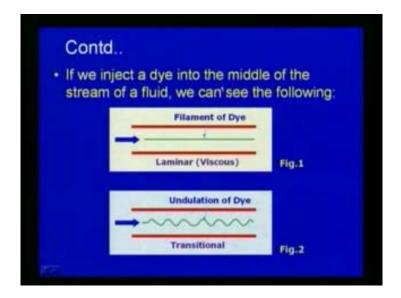
So now, say this we can easily visualize. Say in a pipe flow, if we inject a dye in the middle of the stream of fluid, say if it is fully laminar, you can see that in the slide, so, this is the pipe and pipe the flowing fluid is there, and then, if we inject some dye at the middle, then you can see that the flow is laminar, then you can see there will be a filament of dye like this and it is say flowing like this just as symbol layers. So then, we say that the flow is laminar.
