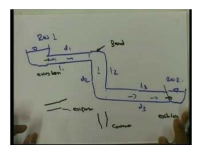
Say for example, if we consider a pipe flow like this say from say one reservoir to another reservoir or one tank to another tank like this, so, here, one of the important aspect is say when we discuss the pipe flow, the flow is taking this direction. So, we can
