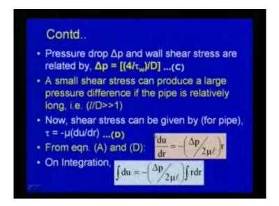
And then, from our early equation c which is here, say this equation delta p is equal to 41 tau w by D. We can write u r is equal to, if you substitute for tau w with respect to the tau w, we can write u r is equal to tau w into D by 4 mu into 1 minus r by R whole square, where capital R is the radius of the pipe. So, here D is the diameter of the pipe; capital R is radius of the pipe. So, we get the velocity as a relation between the wall shear stress and the diameter or the radius of the pipe.
