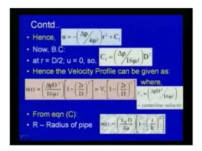
So, hence, we can derive a relationship for the velocity as u is equal to minus delta p by 4 mu 1 into r square plus C 1. So, here, this C 1 is the constant of integration. So, finally, we got the relationship for the velocity.
