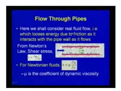
So now, first, we will discuss in detail about the laminar flow systems in pipes, and then the turbulent flow systems in pipes, and then we will discuss about the losses in pipes - major loss and minor loss.
