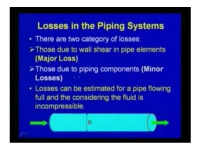
So, like this, we can classify the losses in to major losses due to the wall shear, and then, the due to the minor losses, due to the piping components like bends or the entrance or exit or the junction or the expansion or contraction. So, losses can be estimated for a pipe flowing full, and consider the fluidity is incompressible, so, most of the fluid which we consider in all our discussion is incompressible fluid flow.
