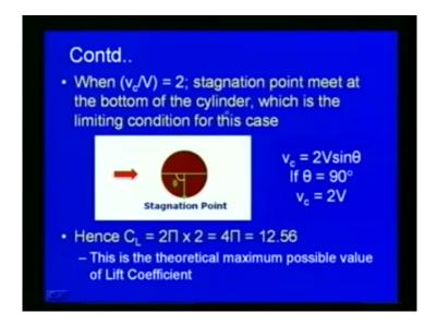
So, now, you can see that, when we analyze various cases, when this v c by V is equal to, you can see that stagnation point meet at the bottom of the cylinder, as in this case here, which is the limiting condition for this case. So, we have already seen this v c, that means, the velocity on the periphery of the cylinder, v c is equal to 2V sine theta, and this will be maximum when theta is equal to 90 degree. So, if theta is equal to 90 degree, we can write v c is equal to 2 into V.
