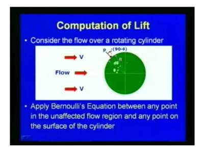
So, we can write the pressure at any point on the cylinder here, at any particular point p, so, if we consider the p 0 as the pressure outside the cylinder which is not affected, so that we can see here, p is equal to p 0 plus half rho capital V square minus half rho small
