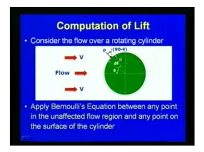
Now, we lift dF L on an elementary surface area of the cylinder, so, if you consider, in the previous figure here, if you consider the elementary surface area, then we can get this, this dF L can be written as dF L is equal to minus LR d theta delta p sin theta.
