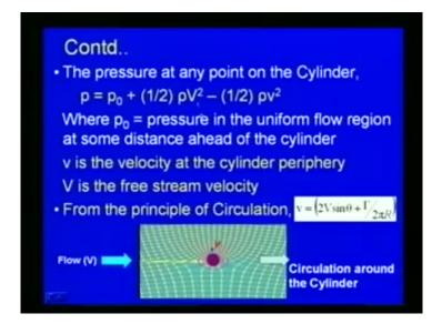
So, this case; so, the pressure at any point on cylinder, we can derive as, p is equal to p 0 plus half rho V square minus half rho small v square, where rho p 0 is the pressure in the uniform flow region at some distance ahead of the cylinder, and small v is the velocity at the cylinder periphery, and capital V is the free stream velocity.
