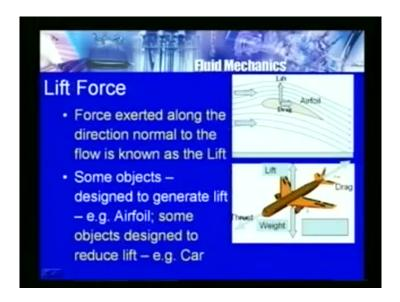
So, as I mentioned, for an aircraft is concerned, you can see that the thrust is in this direction and drag is here, and then weight of the aircraft and lift is in this direction, which is, say, here. We are generating this lift, so that the aircraft is going up and flying. But as far as car is concerned, you can see that, since with respect to the lift, the efficiency of the vehicle will be reduced; so, we want to reduce the lift.
