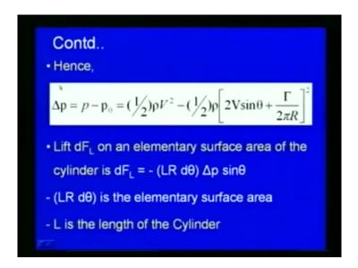
So, this LR, where L is the length of the cylinder, so, R is the radius of the cylinder, LR d theta is the elementary surface area and we will get the lift on the elementary area as dF L is equal to minus LR d theta delta p sin theta; so, we can see here, with respect to this
