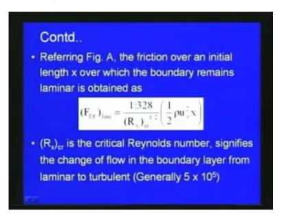
If you refer to this figure where this length of the transition for laminar starts as far as this length is concerned, the friction over an initial length x over which the boundary remains laminar is obtained as  $F_{DF\ laminar}$  is equal to 1.328 by  $R_{X\ critical}$ , critical Reynolds number to the power 1 by 2 into 1/2 rho u infinitive square into x, where u infinitive is the free stream velocity,  $R_{X}$  is the critical Reynolds number at that location. That means at x the
