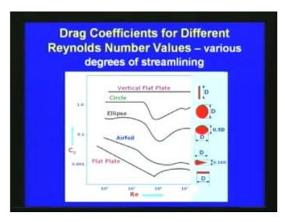
In this slide the drag coefficient for different Reynolds number values are plotted for various shapes.
