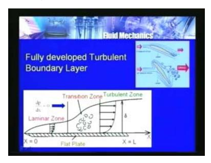
We have calculated the coefficient of drag and various other parameters as we have seen here. We were discussing about the flow over a flat plate. We have seen that initially there is a laminar zone and transition zone and then we were discussing about the turbulent zone.
