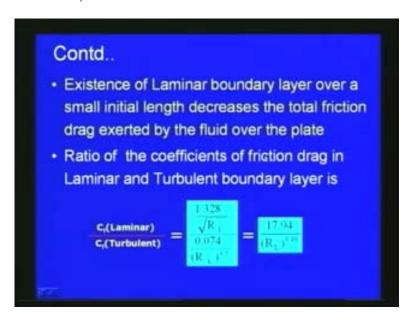
For this kind of problem, the existence of laminar boundary layer over a small initial length decreases the total friction drag exerted by the fluid over the plate. As we can see initially the length of the plate in such a way that there is a laminar boundary layer exists. This existence of the laminar boundary layer over a small initial length actually decreases the total friction drag exert by the fluid over the plate. If you consider the ratio of the
