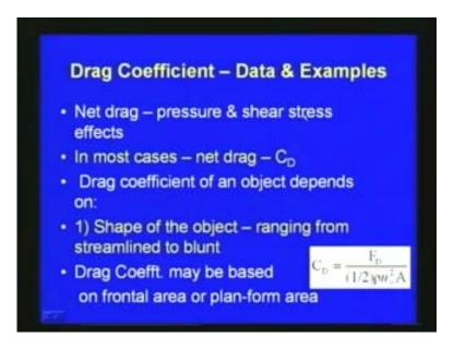
Now, here we discuss the drag coefficient data and examples. Net drag, as we have seen net drag is coming from the pressure drag and the shear stress effects. In most cases net drag we represent as  $C_D$ ; so, the drag coefficient of an object depends upon various parameters. This parameters depends even what is the shape of the object or which the flow take place or which orientation we put say, even the same body or like depends upon the fluid flow parameters.
