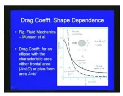
Here, in this slide a graph taken from Munson et al fluid mechanics text book Munson et al. The drag coefficient, based upon the shape dependence of the drag coefficient is plotted here. You can see the drag coefficient for an ellipse with the characteristic area either frontal area that means A is equal to b into D, where b is the length and then D is if you consider an ellipse then this is 1 and here this is d and b is the length or plan form area will be a is equal to b into 1.
