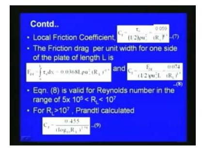
We have seen the local friction coefficient  $C_f$  is equal to 0.059 divided by  $R_X$  to the power 1 by 5 and then from the calculations for the Reynolds number greater than 10 to the power 7 Prandtl calculated the coefficient of drag  $C_f$  as 0.455 divided by  $log_{10}$   $R_L$  to the power 2.58.
