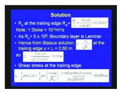
So at the trailing edge means at the end of the plate, so here at this location, so that means the boundary layer thickness here so we can see that L is equal to .6 so delta L is equal to 5 into .6 divide by and Reynolds number square root of 2.25 into 10 to the power 4 which is Reynolds number so we get the boundary layer thickness at the trailing edges 0.02 meter and now the second problem here is the find out the shear stress at the trailing edge.
