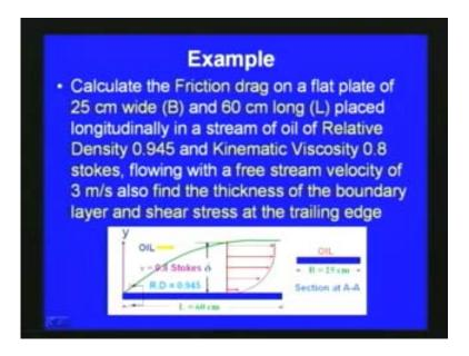
This is the section of the plate, so for this problem we have to find out the thickness of the boundary layer and the shear stress at the trailing edge. We have already seen for these kinds of problem enough for the we can first find out the at the trailing edge what will be the Reynolds number, so that we can see that with respect to the whether the flow is laminar or not and then we can use the equations which we have discussed earlier to get the boundary layer thickness and the shear stress.
