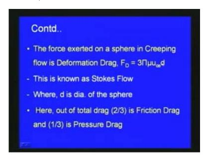
So this known as Stokes flow where this equation is applicable that kind of flow is called as stokes flow and as far as drag is concerned stokes shows that generally this after the total drag two third is the, say in the case of a creeping flow say if we consider the creeping flow over a sphere is shown that two third is friction drag and one third is generally pressure drag.
