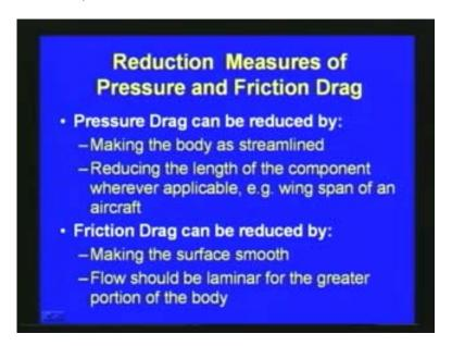
So example, the wing span of an aircraft, we can see that here is the aircraft and then the wing span. Depending upon how you place the wing and then how it is oriented and if you reduce the length component then the pressure drag can be reduced. So like this various measures we can adopt to reduce the pressure drag. Second kind of drag is the friction drag we can reduce the friction drag by making the surface smooth.
