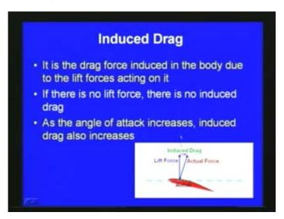
Here we can see that if you consider an airfoil like in this figure here, then we can see that the drag force will be in this direction and then the lift force will be the normal direction of flow direction. Then we can see that since the airfoil is placed with respect to some angle of the free stream flow then we can see that an induced drag will be coming here. So this is due to the lift force.
