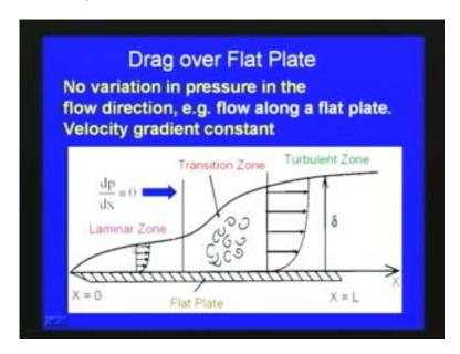
So in this case we can see that here we have the laminar zone and then there is transition zone and here with respect to boundary layer formation we have the turbulent zone. Now with respect to these various cases, we will determine the drag how to find out the drag for a laminar case and then turbulent case and also the transition case.
