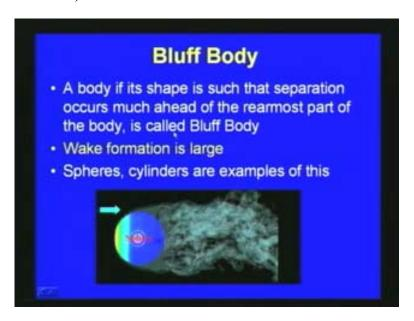
In the case Bluff body say as in the case of a sphere or the case of a circular cylinder we can see that the body shape is such that separation occurs much ahead of the rearmost part of the body. You can see that this is the sphere here, the separation occurs much ahead of the rearmost part of the body. That is why it is called as a bluff body and then you can see the wake formation is large as in the case of a sphere or a cylinder and object
