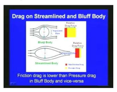
We can see that in the case of bluff body like in the case of a circular cylinder the pressure drag will be much more and then friction drag or skin friction drag will be much smaller and also the total drag will be much higher compare to the streamline body. So the case of an airfoil which is a streamline body, we can see that the skin friction drag.
