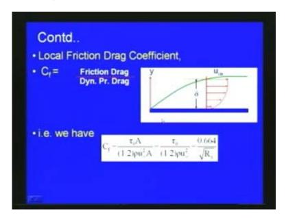
So this  $C_f$  is the local friction drag coefficient for the laminar boundary layer formation over a flat plate. Now the friction drag say over one side of the plate of length 1 per unit width we can write as  $F_{Df}$  is equal to integral 0 to L tow<sub>0</sub> dx, so this is equal to integral zero to L 0.332 divided by u infinitive square root of u infinitive X by mu into rho u infinitive square dx.
