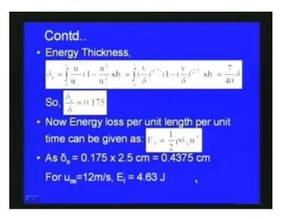
Now, the energy loss per unit length per unit time can be obtained as  $E_l$  is equal to half rho delta e u infinity square. So, delta e, we can substitute as 0.175 into 2.5 centimeter, where delta is 2.5 for the even section. So, this is equal to 0.4375 centimeter, from which
