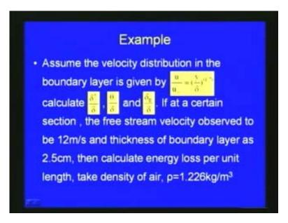
We have to calculate the ratio of displacement thickness to boundary layer thickness, delta star by delta and momentum thickness to delta, and energy thickness delta e to delta. Also, if at a certain section, the free stream velocity observed to be 12 meter per second and thickness of boundary layer as 2.5 centimeter, then calculate energy loss per unit length by taking the density of air as rho is equal to 1.226 kilogram per meter cube.
