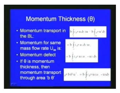
Here, with respect to the flow over a flat plate, which we have seen earlier, say without fluid flow which we consider is b. Then, the momentum transport in the boundary layer we can write as b into integral zero to delta rho u dy into u, where delta is the boundary layer thickness, u is the velocity in the boundary layer, and rho is the density of fluid flow.
