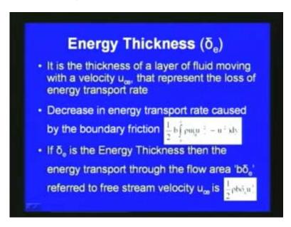
This is with respect to the energy thickness for the flow through area b delta e. Now, we can equate this to the earlier expression and this one, here, so that we can write as half rho b delta e u infinity cube is equal to half b integral zero to delta rho u infinity square minus u square dy.
