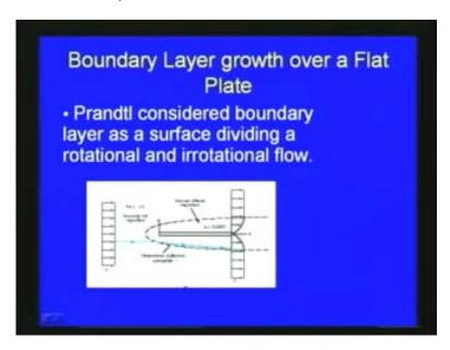
Within the boundary layer, Prandtl considered the fluid flow as rotational and beyond the boundary layer; he considered the flow as irrotational flow. Here, you can see, when free stream velocity is coming over the flat plate, both sides it is shown. So, the boundary layer is developing and then this is the rotational flow free within the boundary layer, both sides of the plate. Beyond this, prandtl considered as irrotational flow.
