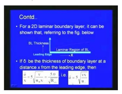
Here, as we have already shown here in this figure, at various locations, this boundary layer for this laminar region, this is x at this distance. So, we can define delta as 5 into square root of new into x by u infinity, which is the free stream velocity and x is at various locations which we considered. This relationship was derived by Blasius through
