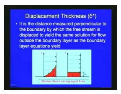
The displacement thickness is defined as a distance measured perpendicular to the boundary, by which the free stream is displaced to yield the same solution for flow outside the boundary layer as the boundary layer equations yield.
