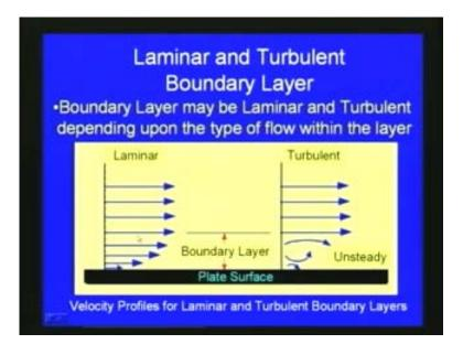
Initially, we will discuss differences between the laminar and turbulent boundary layer. Then, we will see the flow over a flat plate again. Here, in this figure, you can see that this is the free stream velocity coming and then we introduce a flat plate like this. If you plot the velocity profiles for laminar and turbulent boundary layers, we can see that, with respect to boundary layer thickness we have already shown in the previous figure, for a
