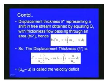
So, this one is with the boundary layer and this is the one without the boundary layer. So, with this, we can see that reduction flow rate by formation of the boundary layer is equal to  $Q_r$  is equal to  $Q_i$  minus  $Q_r$ , so that, we can write this is equal to  $Q_r$  into integral zero to delta  $Q_r$  in integral zer
