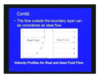
If you flow the velocity profiles for real and ideal fluid flow. So, real fluid, you can see that, due to the no slip condition here, the velocity distribution will be going parabolically like this and then depending upon the flow depth, it is coming here, the maximum. But, in the case of ideal fluid flow, we do not have to consider this no slip condition. So, it is the fluid velocity which will be like this.
