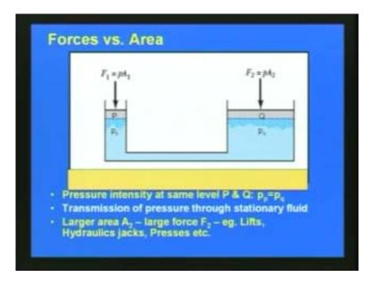
We have seen the application of the concept of force versus area, here as we have discussing the last lecture say here force  $F_1$  on this side is p into  $A_1$  and other side  $F_2$  is equal to p into  $A_2$ . Since p is say on both side is the level p and q.  $p_p$  is equal to  $p_q$ .
