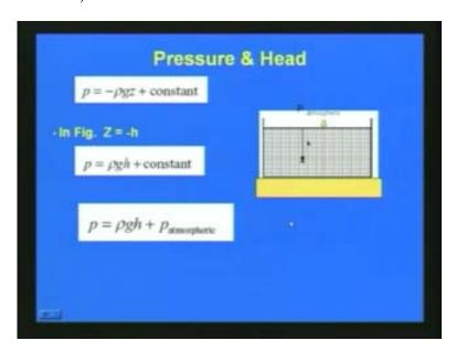
Now, we will briefly discuss the relation between the pressure and head. So for that purpose let us consider say a small basin of fluid or say here water is shown here. Now this fluid this is in static condition the pressure on the surface is atmospheric pressure as here shown in this figure.
