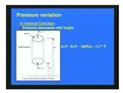
And also we have seen the pressure variation vertical direction and also the horizontal direction.
