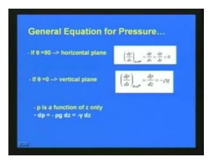
So then the dp by ds is equal to minus row into g, here we can see that this is a small basin where we have stored me water. In the horizontal plane you can see that the pressure is 0 and in the vertical plane you can see that the pressure when theta is equal to 0 and dp by ds is equal to minus row g and here this p, the pressure intensity is a function
