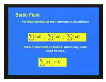
We have seen that the equation sigma  $f_x$  is equal to 0 sigma  $f_y$  is equal to 0 sigma  $f_z$  is equal to 0 at sum of the forces in xyz directions equal to 0 as we use in lid mechanics
