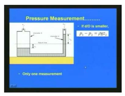
So, this kind of problems if we consider a manometer or this mechanism like this where the diameter d is much larger compared to the diameter D on this line.
