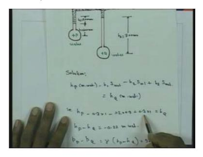
So 0.2 into 9 plus this is again this  $h_3$  is water 0.7 into 1 that gives hq the pressure difference between p and q is hp minus hq is equal to minus 0.22 meter of water this can be we have, we want to get in terms of Pascal.
