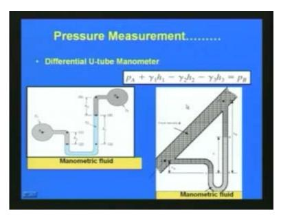
So first one is the last slide just only one limb of the manometer is connected to a particular location where we want to measure the pressure and now if you want to measure the pressure differentially that means between two position say here A and B
