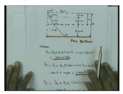
So first layer is about 100 meter and second layer is 200 meter and third layer is 300 meter and this is the sea bed or sea bottom.
