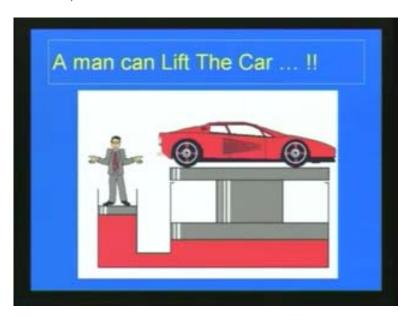
So here car is placed on this side and here is also the man is standing and you can see just with his weight due to application of this principle the car is lifting. So that is very much obvious from this animation. So, what is happening is the pressure intensity same on both sides but here the area is smaller. So with respect to that p into  $A_1$  is much more force using that we can raise this p into  $A_2$  which is very larger force. So, the car is raised as shown in this animation.
