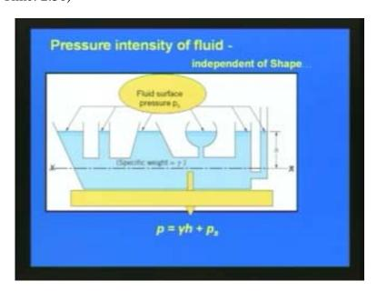
As we have seen in the last lecture, the pressuring density of fluid is independent of shape as we can see here it is on this excess line and then.
