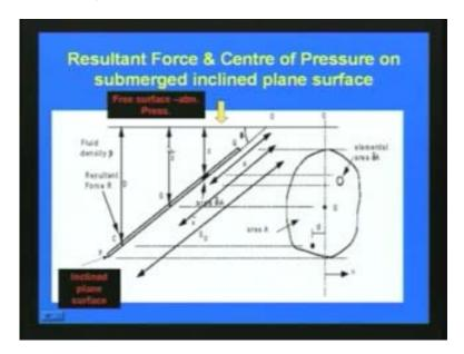
Resultant force and center of pressure on submerged inclined plane surface here this inclined plane surface say here you can see this is a tang of water and then an inclined plane is considered like this and now we want to determine the resultant force and center of pressure on submerged inclined plane surface. So this we will discuss in the next lecture.
