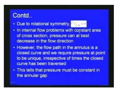
Due to the rotational symmetry we can write del u by del theta is equal to 0 in internal flow problems with constant area cross section pressure can at best decrease in the flow
