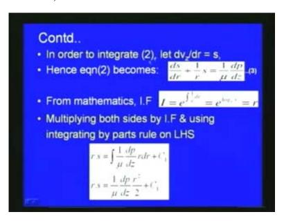
We assume and integration factor if as i is equal to r. We will multiply both sides of equation number three by this integration factor, we will use the integrating by parts rules on the left hand side of this equation finally multiplying by the integrating factor if given i is equal to r using the integration by parts, we can write this equation number three as r
