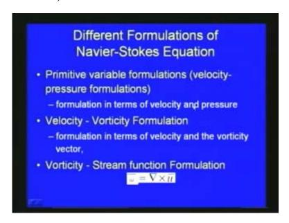
That is what we have discussed and we have derived earlier here the formulation is in terms of velocity and pressure the equations the navier-stocks equations are in terms of the velocity and pressure. These primitive variables are used like velocity and pressure that is why the formulations are called primitive variable formulations. Second kind of generally used the formulation is called velocity vorticity formulations.
