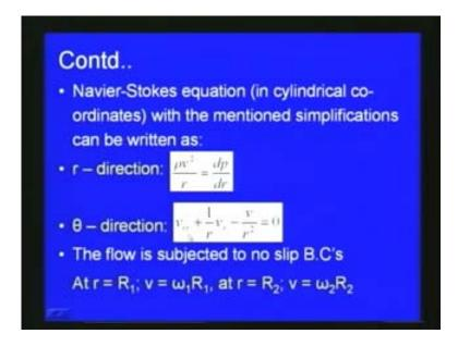
Vary plus 1 by r vr minus v by r square is equal to 0 the flow is subjected to no slip boundary condition that we can write at r is equal to  $r_1$  v is equal to omega 1  $r_1$  and at r is equal to  $r_2$  v writ V is equal to omega 2, these are the boundary conditions for this
