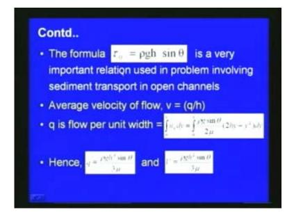
This is a very important relation used in your problem like sediment transport in open channel. Using this expression, we can see how settlement of the sediment takes place sediment transport in open channel we can use this expression if you want to find out the average velocity of flow for this particular problem v is equal to q by h where q is the flow per unit width flow per unit width q is equal to integral 0 to h  $u_x$  dy.
