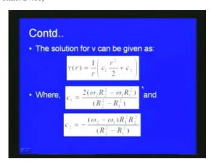
Once we get the velocity we can find out various parameters like shear stress on the wall and other parameters, what we derive for the concentric cylinder problem, the velocity expression mu directly utilized for the viscometer which we have already seen here for the torque can be measured by a torsion wire.
