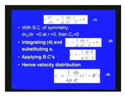
That in this from this equation number four, we will get  $c_1$  is equal to 0 then integrating this equation again and substituting s, as we have already seen and we get vz is equal to 1 but mu dp by dz into r square by 4 plus  $c_2$  as in equation number 5, again here the  $c_2$  we can find out by using the boundary condition at r is equal to r we have the velocity is 0 that we will get  $c_2$  is equal to minus 1 by mu dp by dz into r square by 4.
