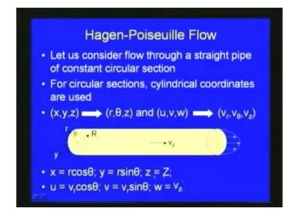
Let us consider the flow through a straight pipe of constant circular section. We can see here is a pipe section this is long pipe and the radius is r capital r for the circular section. As we have already seen we have seen in the navier-stocks equations two forms one is the cartesian coordinate forms and second one is the cylindrical coordinate forms pipe is consigned, we are dealing generally we are dealing with the radius length of the pipe and the angles with which we consider.
