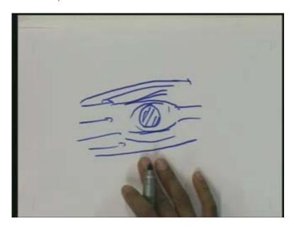
For example: let us consider a cylinder like this flow is coming in this direction. Hence see that away from this here near by the cylinder there will be definitely the effect the boundary layer. But away from the cylinder you can see that, there will not be much effect. Near the boundary we have to consider the boundary layer. By solving this kind of problem, if you consider the flow over a cylinder like this, we can consider the nearby area, we may have to solve the Navier-Stocks Equations.
