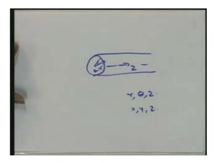
For example: either a pipe flow like this where r is the radius and theta is the angle and z is this direction r theta z here, the coordinate systems are in terms of r theta z instead of x y and z. The velocity components correspondingly, the velocity components are  $v_r$   $v_{theta}$  and  $v_z$ . This equation what we have seen, the Cartesian coordinates equations, we can transform into the cylindrical coordinates in terms of r theta and corresponding velocity  $v_r$   $v_{theta}$   $v_z$ .
