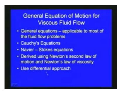
First, we will derive Cauchy's equation the Cauchy's equations are applicable for all kinds of problems compressible and incompressible or work varieties of fluid flow problems and then we will discuss especially we consider the incompressible flow, from the Cauchy's equations we will derive the Navier-Stokes Equation. Here as I mentioned as we have already discussed for the flow between parallel plates here we will use the
