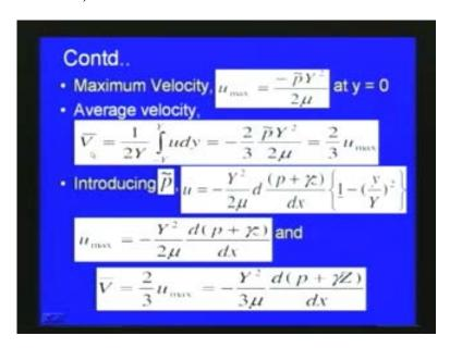
So this is the maximum velocity and then if you want to find out the average velocity V bar is equal to 1 by 2 Y integral minus Y to Y within the limit u dy that is equal to we integrate we can write minus 2 by 3 p tilta Y square by 2 mu, so that we can show that this will be an average velocity will be two third of the maximum velocity.
