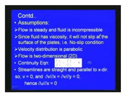
Here the assumptions used are the flow is steady and fluid is incompressible where as the time dependent variables you can neglect since flow is steady and the density variation is not there since flow is fluid is incompressible. Second assumption is fluid has viscosity it will not slip at the surface of the plates that means we consider the no-slip condition. And as we have seen for this particular case velocity distribution is parabolic.
