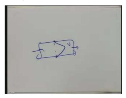
So viscous effect is very important and the corresponding shear stress we have to consider. Viscous flows the shear stress are taken into account and then generally as we have seen in most of the other cases we consider Newton's second law so that we can write the mass of the particle multiplied by the acceleration of particle that will be equal to, we can equate the adequate sum of the forces.
