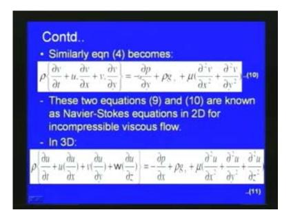
So similar way is z direction rho into del w by del t plus u into del w by del x plus v into del w by del y plus w into del w by del z is equal to minus del p by del z plus rho gz plus mu into del square w by del x square plus del square w by del y square plus del square w by del z square.
