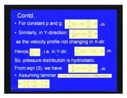
Now here we get an expression with respect to the shear stress, so we can use Newton's law viscosity to convert to get in terms of velocity. So here now the velocity profile is not changing in x direction as we are seen, so hence del tow by del x is equal to 0 that means in y direction is concerned, this equation becomes del by del y of p plus gamma z is equal to 0. So pressure distribution is from this equation number 4, we get the pressure distribution is hydrostatic.
