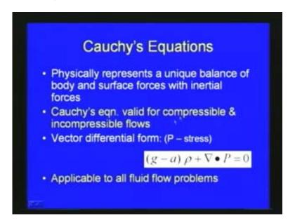
The advantage is depending upon most of the cases which we discussing this fluid mechanism course will be incompressible fluid flow but the Cauchy's equations we can also use for compressible flow also by considering the changing the density also and then here say using the Cauchy's equations only we will be deriving the Navier-Stokes Equation.
