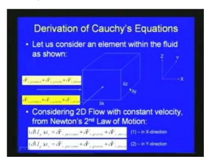
Now let us consider here we derive the Cauchy's equation, so let us consider the element within the fluid as shown here. Here a fluid element of size delta X delta Y and delta Z we are considering. The various forces as we are seen earlier the forces are the pressure force. If you consider this fluid element delta  $F_{x,pressure}$  and delta  $F_{x,gravity}$  the gravity force and delta  $F_{x,stress}$  forces, the stress can be normal stress or shear stresses.
