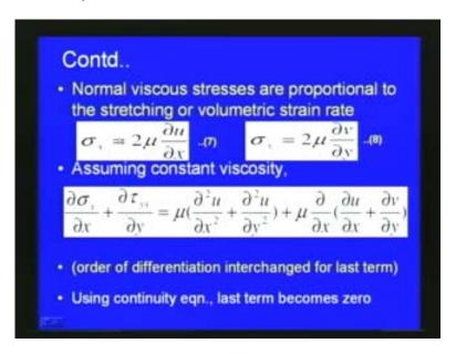
That is why this form is obtained, with respect to x and y the order of differentiation is interchanged and then this term is concerned here we can see that it for two dimensional problems is del u by del x plus del u by del y for incompressible viscous flow this term will be equal to 0. So that finally we get this del sigma x by del x plus del tow $_{yx}$  by del y is equal to mu into del square u by del x square plus del square u by del y square.
