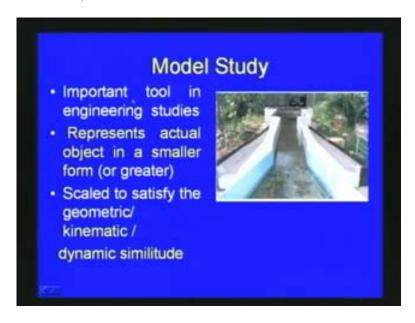
As I mentioned in the beginning this model study is very important. Modeling is an important tool in engineering studies, you can see the model of a sump pump which is in our hydraulics laboratory, a channel open channel, we have done a model corresponding to an open channel and here we provide pump sump you can see this case must done for a
