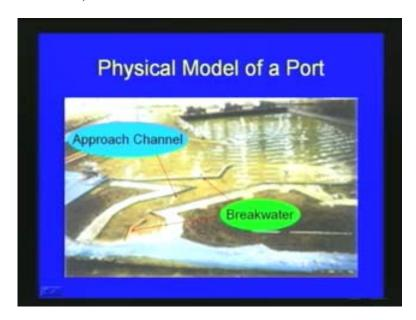
Then, next case is physical model of a port you can see that, the various channels are replicated and breakwater is replicated here in the model appropriate scaling, we can see with respect to a ship comes and if a new construction is made then what happens is waves also will be similar to here and in case tidal effect are there that also simulated in this kinds of model.
