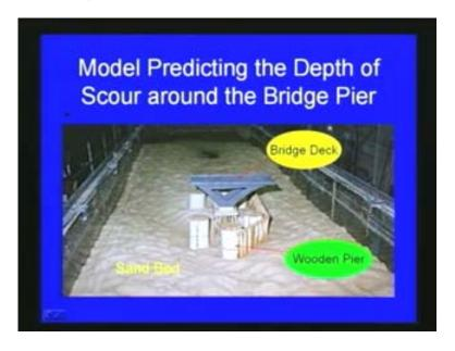
Second case is model predicting the depth of scour around the bridge pier. Here you can see a bridge, a bridge pier is here, this is the channel is there and this sand bed. This modeling is also done based upon the Froude number similarity, you can measure the various parameters with respect to the scour effect on the pier and this is the model with respect to bridge pier covering.
