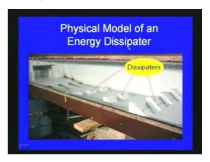
This shows the physical model of energy dissipater energy dissipation, we use the down shade of the dam and you can see all the energy dissipater placed in the model, we will do the simulation.
