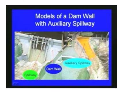
Here this shows the model of the dam wall with auxiliary spillways this also as I mentioned very commonly used, we will doing while before constructing spillways, we will be doing the modeling force spillway this shows how we do for a spillway.
