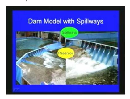
Then, as I mentioned most of the time we will be doing, before constructing a dam spillway we will do physical modeling that is very important since that gives lot of inputs before constructional of the dam or spillways. Here, you can see, we use the Froude number similarity here is the reservoir, the dam with respect to spillway with can construct model going to the appropriate scale this shows a dam model with spillway.
