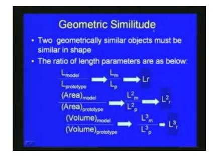
Here you can see that what we are dealing is to geometrically similar objects must be similar in shape, here for example when we deal with the flow over a cylinder you can see that here real field problem will be the diameter will be very large and a cylinder of this glass size is considered, when we do the modeling we consider a small cylinder like this.
