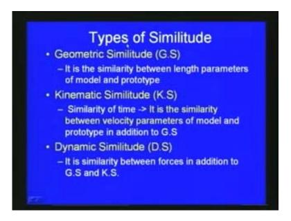
Here the geometric similitude means it is the similarity between the various length parameters of the model and prototype the real field problem which we consider with respect to the length or with respect to the breath or the depth various dimensions of the real field problems, how we model or how we do the similarity this is the geometric means length breadth and depth with respect to this parameters, how the similarities adopted called the similitude is adopted.
