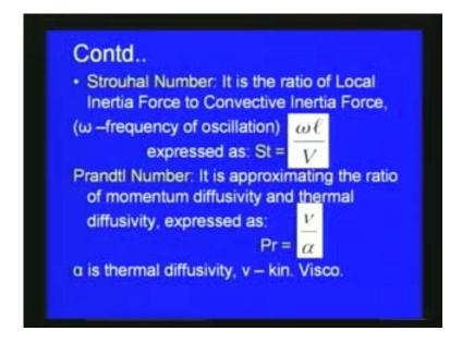
Strouhal number St is equal to omega l by V where omega is the frequency of relation l is the characteristics length and v is the velocity, Strouhal number is the ratio of local inertia force to convective inertia force. Another important number is prandtl number.
