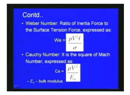
Many fluid mechanics problem surface tension is important here we can use this weber number the dimensional number weber number. O this Weber number is defined as rho v square 1 by sigma where rho is the density of the fluid v is the velocity 1 is the characteristic length and sigma is the surface tension force.
