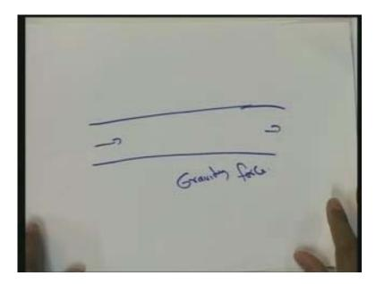
It is the ratio of inertia force to gravity force and it is expressed as the froude number Fr is equal to V by root gl where, l is the characteristics length it can be depth or it can be various other parameter, depending up on which may be other dealing the problem it is the froude number FR is equal to V by root gl or l can be in the case of open channel flow t can be depth of flow.
