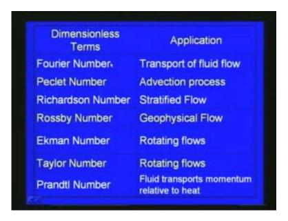
With the transport of fluid flow there in that case Fourier number is important and we use the Fourier number peclet number. As I mentioned this shows the advection defuses process especially advection process is important there we use the peclet number.
