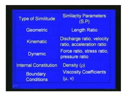
Finally, when we do the similarity parameters are the length ratios and kinematic similarity parameters are the discharge ratio velocity ratio and acceleration ratio.
