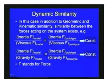
Similarity between the forces acting on the system exist inertia force of the model divided by viscous force the model should equal to inertia force the prototype divided by the viscous force of the prototype.
