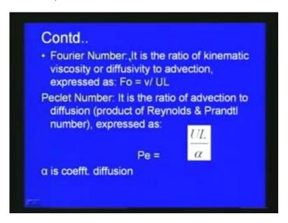
Another important number is called Fourier number dimensions number Fourier number is the ratio of kinematics viscosity of diffusivity to advections, here the Fourier number is defined as mu by UL where v is the kinematics viscosity U is the velocity and 1 is the characteristic length which we consider.
