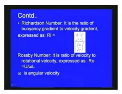
Wherever the buoyancy effect is very important this number is used, Richardson number is the ratio of buoyancy gradient to velocity gradient and this is expressed as Ri is equal to g by rho del p by del z divided by del u by del z whole square, this is the Richardson number. Another important number is called rossby number.
