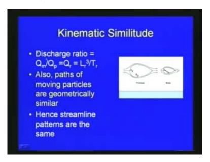
Then you can see the discharge is concern discharge ratio is  $Q_m$  by  $Q_p$  that is the with respect to the stage of the model divided by this state of the prototype that is the ratio that is equal to  $L_r$  cube by  $T_r$  L<sub>r</sub> is the length ratio and  $T_r$  is the time ratio  $L_r$  cube by  $T_r$
