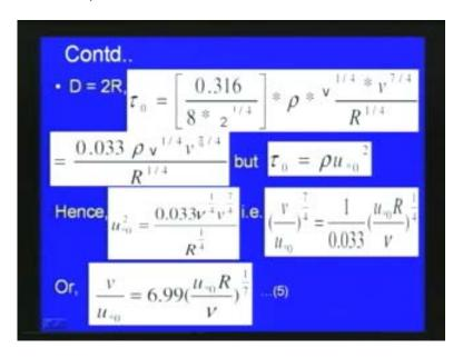
So now, if we substitute for diameter D is equal to 2R and then we will be trying to approximate simplifying this equation. So tow<sub>0</sub> is equal to 0.316 divided by 8 into 2 to the power 1 by 4 into rho into mu to the power 1 by 4 into mu to the power 7 by 4 divided by r to the power 1 by 4 as shown in this slide. So here you can see in this slide the expression for tow<sub>0</sub>.
