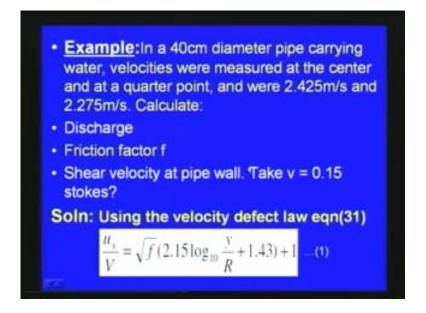
For this problem, the pipe here is for turbulent flow in pipe, this is the central line. The diameter is 40 centimeter. The velocities were measured at the center point as shown here and the velocity at the center point is 2.425 meter per second and then quarter point. So here this is R by 2, at this location velocity is measured as 2.275 meter per second.
