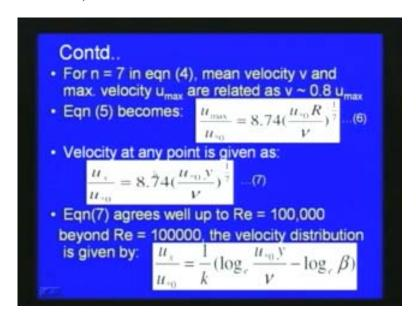
As we have seen, if we use for the power law n is the constant which is varying from 6 to 10 as we have seen, so now if we use here, for particular case say n is equal to 7 then we can see that the mean velocity v and maximum velocity generally, for pipe flow we can write approximate the average of velocity v is equal to 0.8 times the maximum velocity or 80% of the maximum velocity.
