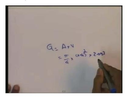
So the discharge through the pipe once the average velocity is given discharge is equal to Q is equal to area of flow section multiplied by A into Q is equal to A into v. So here A is pi by 4, v is 0.4 so pi by 0.4 squared into the velocity average velocity is 2.093 meter per second.
