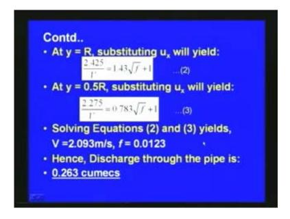
So now at y is equal to R if we substitute you can see that the velocity at the central line is given the maximum velocity is given, so if we put this expression 2.425 divided by v is equal to 1.43. So here R by R, this expression it is 1.43 root f plus 1 so that is equation number 2, similar way the velocity at y is equal to 0.5 R is given, so we can put this in this expression equation number 1. So 2.275 by v is equal to 0.783 root f plus 1 after
