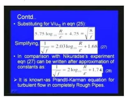
So that here for this u star o by v with respect to this expression we can substitute back so substituting for v by u star o in equation number 25 we can get 5.75 log 10 R by epsilon plus 4.75 is equal to square root of 8 by f.
