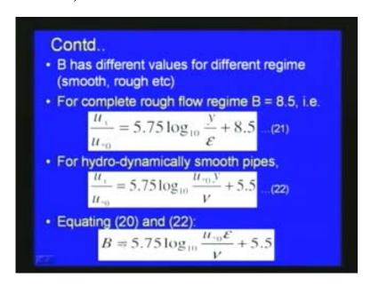
Now, this constant we have seen this constant B has different values for different regime, as we have already seen whether the pipe is rough, smooth or between which range there value of B changes. So for complete rough flow regime we can show that B is equal to 8.5, so that we can write  $u_x$  by u star o is equal to 5.75 log 10 y by epsilon plus 8.5 as in equation number 21.
