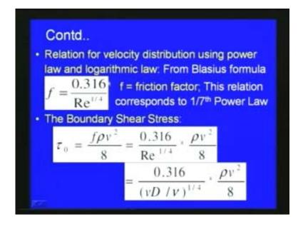
Now our aim is either by using power law or the logarithmic law we want to derive the velocity distribution expression for turbulent flow in smooth pipes. Now if we consider the boundary shear stress, sotow<sub>0</sub> is equal to f rho v squared by 8 where rho is the density of the fluid; f is the friction factor; v is the average velocity.
