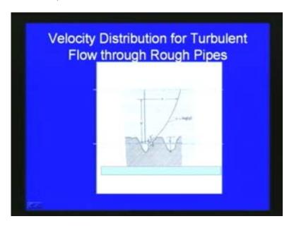
We can see these are rough type pipes. We can see here initially variation is for the sub layer which we consider the variations is like this either it is you can see linear or we can approximately using the power law and then after that laminar sub layer, we can see that we will be approximating the expression with respect to the logarithmic law or v is proportional to the average velocity v is proportional to logarithmic law of y.
