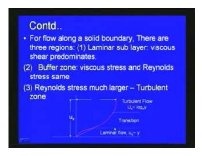
So this is the transition of buffer zone and then the turbulent zone. We can see that the Reynold's stress have larger and then here you can see that the velocity is proportional to the natural logarithmic of the distance y as shown here. These are the variations with
