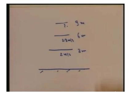
So if the meteorological station here, you can see that if this is the ground level, here we have 3 meter then 6 meter and 9 meter. Here, the velocity is given as 2 meter per second here 2.3 meter per second. So we have to determine the velocity and this 9 meter location.
