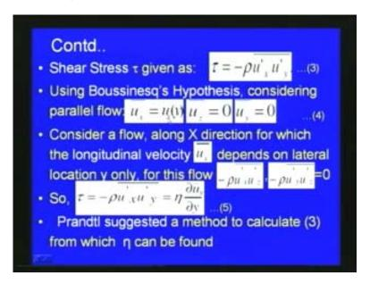
What he considered here is we can see it is a parallel flow, so in the parallel flow case for example, if we consider plate like this and then he considered parallel flow, such that for this particular case the velocity variation, if this is x direction and here this is y direction so that x variation is with respect to  $u_x$  and y only and other components like the z component and the y component are 0.
