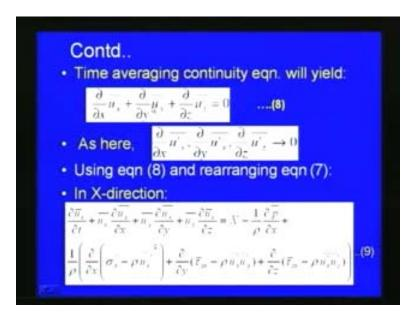
If we use the time averaging concept for the continuity equation we can write the continuity equation as del  $u_x$  bar by del x plus this equation slide here plus del by del y  $u_y$  bar plus del by del z  $u_z$  bar is equal to 0 equation number 8. Here you can see that as far as some of the other terms are concerned this we have discussed earlier del by del x of  $u_x$  dash bar and del by del y of  $u_y$  dash bar and del by del z of  $u_z$  dash bar tends to 0.
