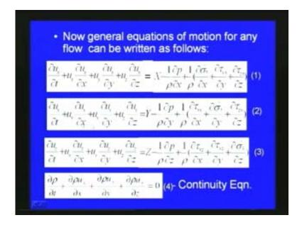
Now, the general equations of motion, so called Cauchy's equation we can write as I mentioned this equation we will be discussing later in the nevier stokes equations in chapter. This equation in x y z component we can write as del  $u_x$  by del t plus  $u_x$  into del  $u_x$  by del t plus  $u_y$  into del  $u_x$  by del t plus del t
