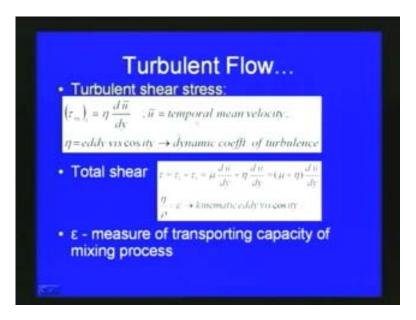
Now another important parameter is turbulent shear stress. So turbulent shear stress we can express as tau x y with respect to t that is equal to eta d u bar by dy, where u bar is the temporal mean velocity. We have already seen what temporal mean velocity is. That means with respect to the long time how the variations take place for the mean velocity. The turbulent shear stress we can express as eta into d u bar by dy, where eta is called the eddy viscosity or dynamic coefficient of turbulence.
