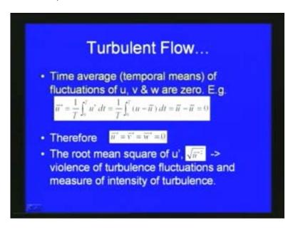
We have seen the time average of this fluctuations u v w are 0 since we can show as we have seen earlier the mean component of u dash is equal to 1 by T integral 0 to T u dash dt that can be equated to 0, similarly v and w also. Generally, we express this root mean square u dash bar whole squared that gives to describe the violence of turbulence fluctuations and it is generally a measure of intensity of turbulence.
