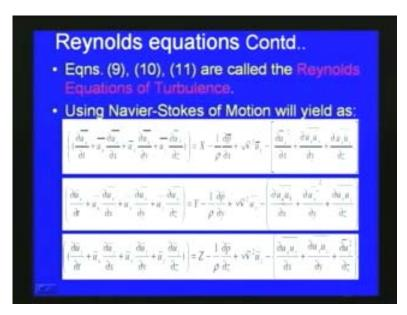
Here, as far as the turbulent flow is concerned now the basic equations here are the Reynolds equations of turbulence equations 9, 10 and 11 as we have already seen here equation 9, 10 and 11. So these equations are called the Reynolds equation turbulence which is the basic fundamental equations of turbulence.
