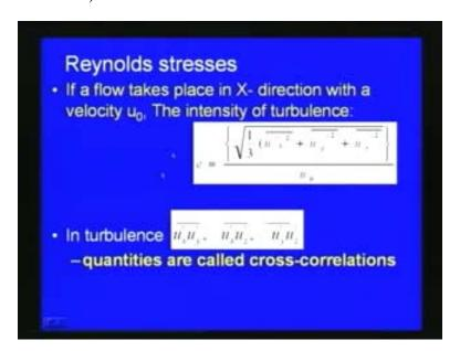
We have already seen the intensity of turbulence is expressed as e is equal to square root of 1 by 3  $u_x$  dash bar square  $u_y$  dash bar square plus u  $w_z$  dash bar square by  $u_0$ , where u 0 is the mean free mean the free stream velocity and says these quantities like  $u_x$  dash  $u_y$  dash bar  $u_x$  dash  $u_z$  dash bar  $u_y$  dash bar. These quantities are called cross correlations.
