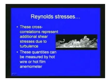
So what we do? As I mentioned turbulent flow solution is very difficult since the variations, so many unknowns and then we have got only few equations. Generally, use a theory, statistical theory so there we use this mean flow mean component, then RMS and then the cross correlations.
