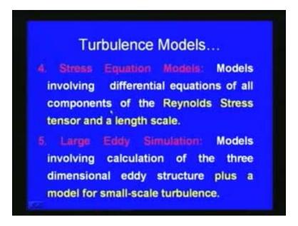
Forth kind of equation model is called a stress equation model. Here, the models involving differential equations of all components of the Reynolds stress tensor and a length scale. So this is called stress equation models, where we use all the differential equations and components of the Reynolds stress tensor and a length scale.
