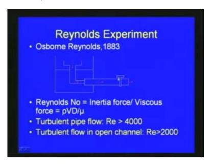
And then fitted a pipe here and then with respect to time he put valve here. As we can observe when the valve is opening, initially this is here, you can see when the valve is opening a filament of dye is passing through the flow is very much laminar in nature; then we can see that after some time the flow is transitional stage when the valve opening is increased then you can see small disturbance starts and then it becomes finally total turbulent flow.
