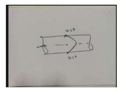
So, due to the no slip condition on the pipe boundaries the velocity will be 0 on the pipe valve; then we can see that the pipe velocity will be maximum at the center; then again say other side it will be 0. So with respect to this we can now bring the velocity variation for the laminar flow in pipes we can just here in this slide we can see that the velocity is varying, the velocity variation is here.
