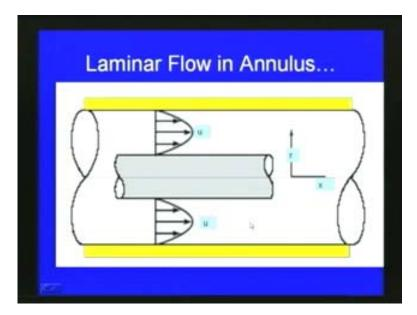
This location, this location and this location that means on the pipe valve here you can see work place the velocity is 0 and then it is going. Here, at this line it is the maximum velocity this is the velocity u and similarly here also very similar way we can plot the velocity here the minimum on both sides and here the maximum velocity.
