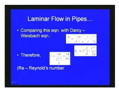
Darcy-Weisbach equation is given as f L v square by 2 g d, where f is the friction coefficient for the pipe, L is the length of the pipe, d is the diameter, V is the average velocity, and g is the acceleration due to the gravity. Therefore we can write the friction coefficient f is equal to 64 divided by rho v d by mu that is equal to 64 by Re, where Re is the Reynold's number.
