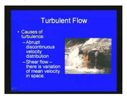
The flow is coming and then due to various parameters various factors discontinuity takes place you can see here these rock is here and then the flow is coming various obstructions are there and then due to this the velocity become discontinuous or discontinuous velocity distribution takes place, this can be one of the major cause of turbulence and
