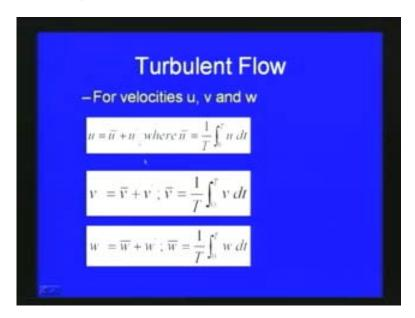
Long time is considered, so 1 by t integral 0 to t u dt and V turbulent velocity direction v is equal to v bar plus v dash so where v bar is equal to 1 by T integral 0 to t v dt. Similarly w is equal to w bar plus w dash, where w bar is equal to 1 by T integral 0 to T w dt, where u dash v dash w dash are the instantaneous velocity with respect to mean velocity as we have discussed.
