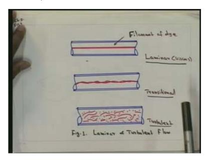
This is the laminar flow and turbulent flow which we have discussed in the beginning of this chapter. Now we are going to discuss more on the turbulent flow as we have already covered the laminar flow at steady state. Now we will be discussing the turbulent flow so the laminar to turbulent as we have seen it is through a transitional stage.
