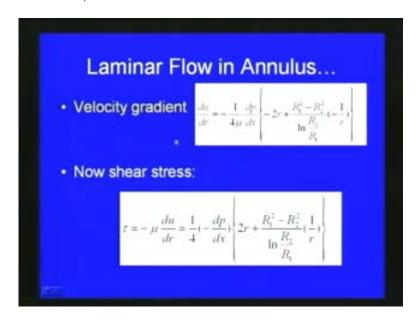
So this gives the shear stress. As we have plotted the velocity variation in the case of pipe flow here also we can plot the velocity variation, I mentioned due to the no slip boundary conditions on the pipe valve as well as the inner cylinder of valve, the velocity will be 0, so we can see here I have plotted the velocity variation here.
