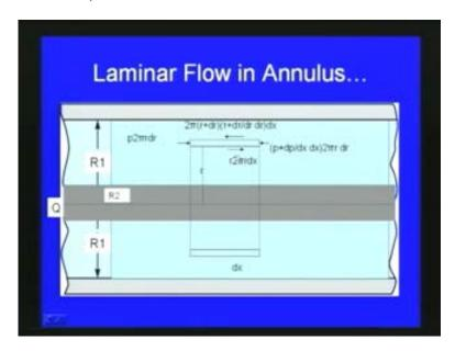
This is the inner cylinder and this is the outer cylinder and flow is between these two cylinder the flow is direction is like this, like this; then to derive an expression for the velocity variation and discharge the parameters here we consider fluid element like this at a distance r from the central line and the length of the fluid element is dx and then we can see that the size dx by dr is considered and the forces acting here are the pressure force and shear force.
