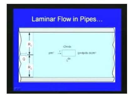
Here, you can see the radius of the pipe is  $R_0$  and Q is the discharge and then we consider a fluid element like this. Using this concept only we have derived the basic equation for the velocity in a pipe flow from the fundamental principles so u is equal to minus 1 by 4 mu into dp by dx into  $R_0$  square minus r square, where  $R_0$  is the radius of the pipe, p is the pressure, mu is the coefficient of dynamic viscosity.
