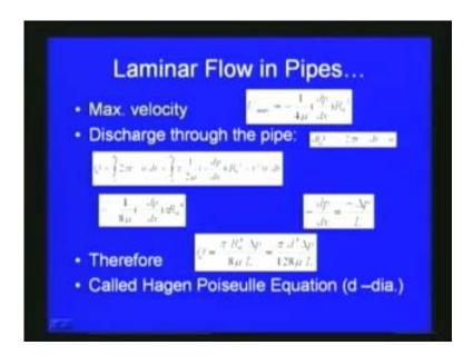
We can see at the center will be the maximum velocity so that is obvious for pipe flow and then the expression for maximum velocity will be in the previous case if you put small r is equal to 0 we get  $u_{max}$  is equal to 1 by 4 mu dp by dx into  $R_0$  square and then very similar way discharge through the pipe we can get dq is equal to 2phi r dr into du.
