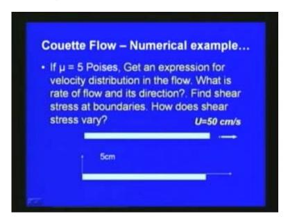
We have to find if the coefficient dynamic viscosity is given as mu is equal to 5 poises we have to get an expression for the velocity distribution in the flow and what is the rate of flow that means how much the discharge passing and its direction? Find shear stress at boundaries. How does shear stress vary?
