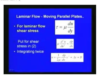
If you integrate twice we get mu is equal to 1 by 2 mu dp by dx into y square plus A y plus B, where, A and B are the constant of integration.
