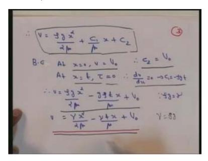
Finally, we can put back the  $C_2$  and  $C_1$  to the expression for the velocity. So, v is equal to rho g x square by 2 mu,  $C_1$  is minus rho g t, so minus rho gt into x by mu plus  $C_1$  is 0. So this is the expression for the velocity which can be simplified as v is equal to rho g is equal to gamma is equal to rho g. We can write v is equal to gamma x square by 2 mu minus gamma t into x by mu plus  $v_0$ . So this is the expression for the velocity.
