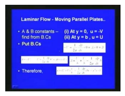
Here again we have got two boundary conditions. As I mentioned here the plates are moving with the velocity so here on the upper plate we know the velocity u is equal to U on the top of the plate and bottom of the plate v is equal to minus V in the other direction.
