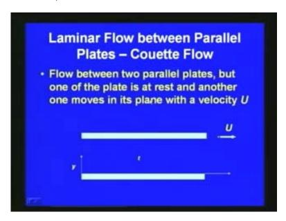
You can see in this slide the flow between two parallel plates but one of the plates is at rest and another one moves in its plane with a velocity u.
