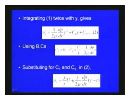
If we integrate twice with respect to y gives  $u_x$  is equal to 1 by 2 mu dp by dx y square plus  $C_2$  y plus  $C_1$  where  $C_2$  and  $C_1$  are constants of integration then we can use this both boundary conditions as we have seen here the boundary condition here u is equal to 0 at t is equal y is equal to 0 that is one boundary condition.
