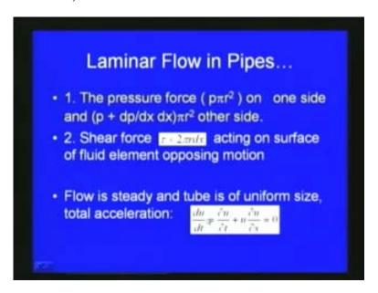
Here, the forces are the pressure force p into phi r square on one side and p plus dp by dx into dx into phi r square on other side. And then the shear force is tow into 2phi rdx acting on surface of the fluid element opposing the motion with respect to the shear force. As we have already assumed the flow is steady and tube is of uniform size; total acceleration is equal to 0 that we can write, du by dt is equal to delt u by delt t plus u into
