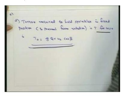
If we want to find out the torque required to hold the sprinkler in fixed position to prevent from rotation, we can write T is when omega is equal to 0, so we can write  $T_0$  that is the torque required to hold sprinkler in fixed position  $T_0$  is equal to rho Q r  $u_2$  cos beta.
