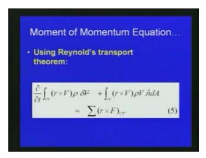
Earlier, we have seen the Reynold's transport theorem. We have already discussed the applications of Reynold's transport theorem, in many problems it is used to derive the basic equations. If we use the Reynold's transport equation to derive the final equation for the moment of momentum equation, we can write with respect to the previous equation number 4.
