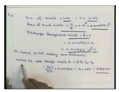
We saw this problem by using the moment of momentum equation or principle, which we have derived in the case of sprinkler system or general system which we have seen. Here, the diameter nozzle is given as 10 millimeter and velocity is given as 12 meter per second; area of each nozzle we can calculate pi by 4 into 0.01 square that will give the value of the area each nozzle as 0.0000785 meter square and then we can find out discharge through the nozzle since the velocity is given.
