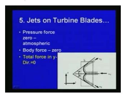
Now again this case all here this particular all we do not consider the pressure force the pressure force is here it is atmospheric pressure or this 0. We consider the pressure force as 0 also the body force is not to be considered here this particular case due to the specific nature of the problem.
