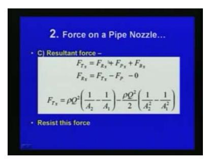
We have already found here., finally, we get the resultant force for the system  $F_{Tx}$  is equal to  $F_{Rx}$  plus  $F_{Px}$  plus F B x and finally,  $F_{Rx}$  is already can be written as  $F_{Tx}$  minus  $F_{Px}$  minus 0 this is with respect to the  $F_{Rx}$  is obtained like this now finally,  $F_{Rx}$  is equal to rho Q square into1 by  $A_2$  minus1 by  $A_1$  here which is obtained from the total force which we have already found  $F_{Tx}$ .
