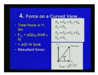
Finally, we get  $F_{Tx}$  in the x direction finally, we can get  $F_{Rx}$  that means the resultant force plus the pressure force any way not considered here body force is al in the x direction there is no body force.  $F_{Tx}$  the resultant force  $F_T$   $F_R$  x is equal to  $F_{Tx}$  here this with respect to the y direction  $F_{Ry}$  is equal to  $F_{Ty}$  minus F B y and the resultant force we can we find out the resultant is equal to square root of  $F_x$  square plus  $F_y$  square.
