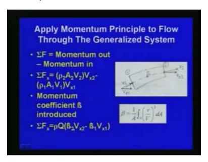
Where this sigma F x is the total force acting upon the control volume external force on the control volume that is equal to the linear moment change with respect to system this we have seen where beta is the moment coefficients correct or moment correction factor as we have seen.
