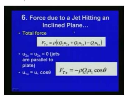
Finally, this expression become since  $u_1$  x is equal to  $u_1$  cos theta this angle is theta  $u_1$  x is equal to  $u_1$  cos theta finally, we simplify the equation to  $F_{Tx}$  the total force in the x direction is equal to minus rho  $Q_1$   $u_1$  cos theta.
