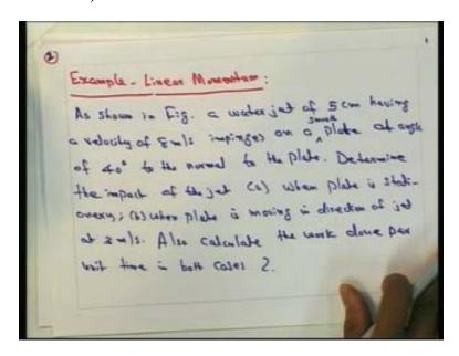
The problem is we have we have a plate put at an inclination of 40 degree with respect to the horizontal that a jet is acting jet is hitting or impinging on the plane at 40 degree.
