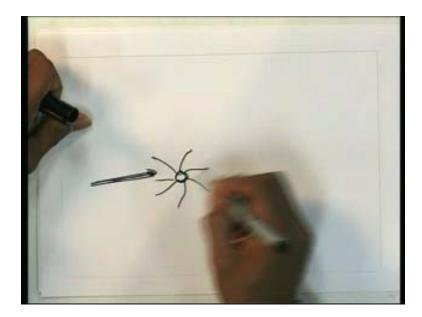
You can see that due to the jet action it is it will start rotating. It is we can use this principle of the linear moment equation which we have seen here we can use the same principle to analyze the impacts of jets on turbine blades.
