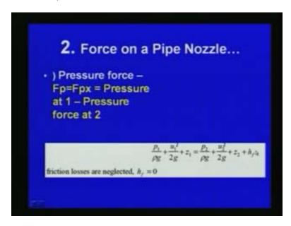
Where  $h_f$  is the losses due to friction here if we neglect the friction losses here then  $h_f$  is equal to 0 that we can write the pressure force from the Bernoulli's equation if we consider this particular case z the data head is  $z_1$  is equal to  $z_2$ .
