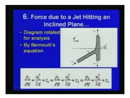
Here the diagram is rotated for analysis now we can see this is angle theta and  $u_1$  is the jet velocity is  $u_1$  and now x is horizontal and y is vertical direction and  $u_3$  is the velocity downward  $u_2$  is the velocity upward.
