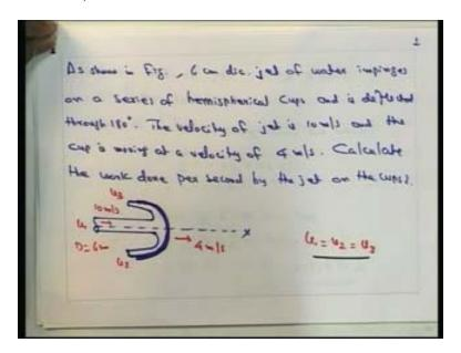
You can see that the jet is coming this direction and the cup is or the vane is placed curved vane is placed like this and it moving the cup or the vane is moving with a velocity of 4 meter per second. The jet velocity is 10 meter per second and if  $u_1$  is the jet velocity then you can see that it will be after the jet reaches the cup it will be deflecting at 180 degree.
