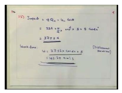
This is the work done, like this we can solve most of the problem by considering the linear moment equation for either a fixed control volume or for a moving control volume.
