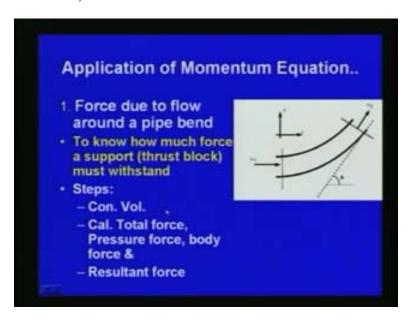
We will be considering as basic steps the basic steps involved or we will be considering control volume, we will be calculating the total force on the system and including the pressure force body force we will be finding the resultant force. We will be equating with respect to the moment change that is what we have seen and we have derived the equation for one of the example force due to flow around a pipe bend in the last lecture.
