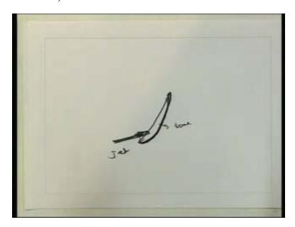
This is the vane here and this is the jet we want to find out how much is the force acted upon acted by this jet on this vane or the curved vane we consider, here for this particular case similar to the pipe pressures here similar to the pipe here the pressures are equal.
