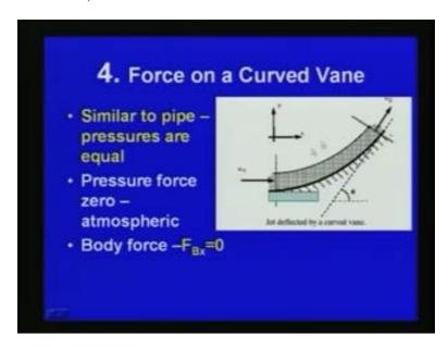
In this slide you can see a jet is coming it is deflected by a curved vane like this, this is the vane here and jet is coming like this here the velocity of the incoming jet is  $u_1$  is the velocity. After deflected by the curved vane it is  $u_2$  and x direction is here y direction is here and the angle with respect to the where the velocity  $u_2$  this angle is theta with respect to this slide here.
