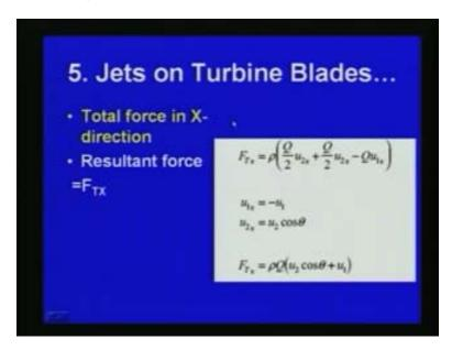
Now the resultant forces obtained as  $F_{Tx}$  here you can see that the  $u_1$  x the velocity we are assign for this particular problem the velocity is coming with respect to the x direction like this in this direction.
