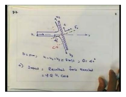
As shown in this figure a jet is hitting on an inclined plate like this we have to find water jet of 5 centimeter having a velocity of 8 meter per second impinges on a smooth plate at an angle of 40 degree to the normal to the plate. We have to find out the impact of the jet when the plate is stationery case a and case b when the plate is moving in direction in the direction of the jet at 3 meter per second also calculate the work done per unit time in both cases.
