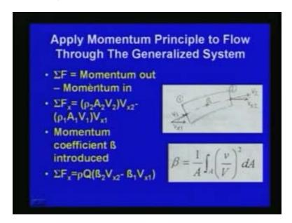
beta<sub>2</sub> is the momentum correction factor at section two and beta<sub>1</sub> is momentum correction factor at section one we can write sigma  $f_x$  is equal to rho q beta<sub>2</sub>  $v_{x2}$  minus beta<sub>1</sub>  $v_{x1}$  this in the x direction similar way we can write the equation in y direction.
