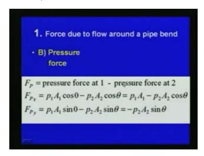
Similarly in y direction we can write the pressure force in y direction  $p_1$   $a_1$  sine 0 minus  $p_2$   $a_2$  sin theta sine 0 is 0 this is equal to minus  $p_2$   $a_2$  sin theta if you consider the body force here mainly it is due to gravity.
