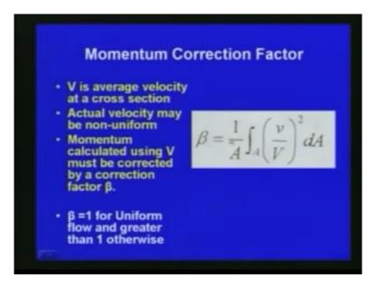
This beta as we have already seen in the case of energy correction factor we can in a very similar way we can derive this momentum correction factor beta as beta is equal to one by a integral a v by capital v whole square where capital v is the average velocity and small v is the velocity at any section which we consider as shown here this is small v and capital v is the average velocity which we consider for the case.
