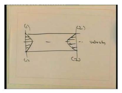
As we have already seen in the case of energy equation and the Bernoulli's equation we have applied a energy correction factor. We are discussing the momentum equation linear momentum equation for the momentum also since we are considering the average velocity at the section we have to apply the apply a correction factor called momentum correction factor momentum calculated using the average velocity must be corrected by a
