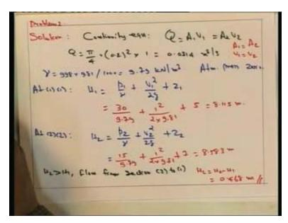
If you consider similar way the section two which we consider here for section total head  $h_2$  is equal to  $p_2$  by gamma plus  $v_2$  square by 2 g plus  $z_2$   $p_2$  is given as the pressure is section two is given as 15 kilo Pascal  $p_2$  by gamma is 15 by 9.79 plus  $v_2$  is 1, 1 square by 2 into g 9. 81 plus  $z_2$  is 7. This we get as 8.583 meter here you can see this  $h_2$  is greater than  $h_1$  since 8.58 there is greater than 8.115 the flow occurs from section two to one.
