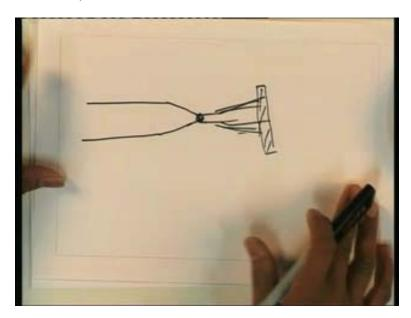
This jet action all the force is exerted by the moving fluid the moving fluids exert forces here we can see here there is a nozzle is there and jet is put on a plate like this, you can
