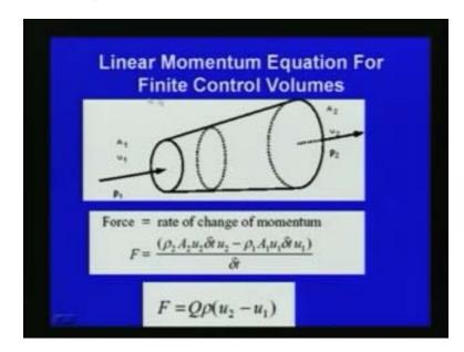
On this section we consider two sections here at this section if the area of cross section is a one and the velocity is  $u_1$  and the density is rho 1 at section two if the area of cross section is a two the velocity is  $u_2$  and the density is rho 2.
