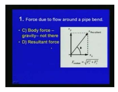
This gives the  $f_x$  force in x direction y direction will be f t y the total force in y direction is equal to rho q  $u_2$  sin theta pressure force in y direction is minus  $p_2$   $a_2$  sine theta.
