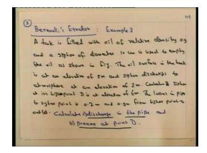
we have to find out the discharge in the pipe and the pressure at point d. problem is here
