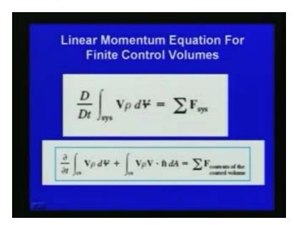
With respect to the Newton's second law, finally, the equation already shown here it is written here d by dt, if you consider the system integral of the system v rho d v is equal to sigma f system you can see the total the adverse me of the forces is equal to the rate of
