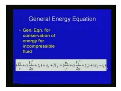
We have already seen considering with respect to two sections of flow between for example if you consider a pipe flow like this, we have already seen here between sections one and two here the total energy equation or general energy equation is written as  $p_1$  by gamma plus alpha  $v_1$  square by 2 g plus  $z_1$  plus q w plus h e is equal to  $p_2$  by gamma plus
