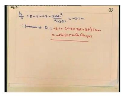
This is the pressure at d like this we can use the Bernoulli's equations for a given problem to find the discharge or the pressure or whatever the variable depending upon the
