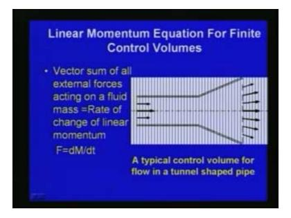
If you consider section between this section and this section we can find out the vector sum of all external forces acting on a fluid mass that will be equal to the rate of change of linear momentum.
