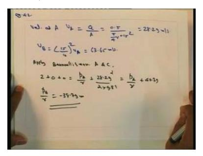
You can see here there is no flow takes place the velocity can be considered as 0 if you consider the Bernoulli's equation between points c and a that, we can find the write the equation as here the  $z_1$  the Bernoulli's equation is applied that will give here the velocity all the values are known this is 2 plus you can see that between this level, the location a and location c the level difference is 2 meter that, we can that 2 plus it is z the location
