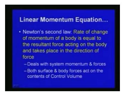
If you consider a open system or closed system the Newton's second law deals with the momentum and the momentum occurring with respect to control volume or the between the sections which we consider and the forces acting on with respect to control volume. As we have already seen the control volume concept.
