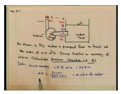
From that we get the head which can take care by the pump that is equal to 4.07 meter of water from that we get the head which can take care by the pump that is equal to 4.07
