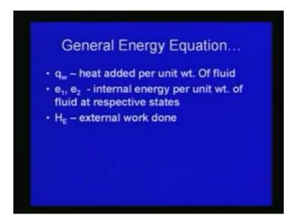
We have already seen this  $e_2$  minus  $e_1$  minus  $e_1$  wis equal to reversible and irreversible, irreversible head is the head loss h l is the energy loss per unit weight of fluid due to the friction and other causes, for incompressible fluid total head at 1 plus heat added due to machine or head loss is equal to total machine minus head loss is equal to total head.
