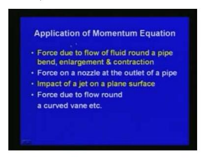
Force due to flow around a curved vane like in a turbine we can use the momentum equation momentum equation which we have derived or which we have seen far has got large number of practical engineering applications. We will be discussing some of the applications here the momentum equations. First one is the application of momentum equation force due to flow around a pipe bend. Here we will discuss a pipe bend here you can see a bended pipe like this here.
