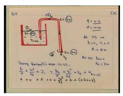
If you consider point one, we can see that here this tank is open to atmosphere that we can say that the pressure  $p_1$  is equal to 0 here the there is no velocity of fluid  $v_1$  is equal to 1 the elevation head is given as  $z_1$  as 5 meter for this problem. At section two where the at the outlet of the siphon, we can see that the pressure is given as  $p_2$  is equal to 0 that it is the flow into the atmosphere  $p_2$  is equal to 0 we can see here the elevation head is given as 2 meter.
