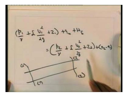
Various terms like q w is the heat added for with respect to the system which we discuss q w is the heat added per unit weight of fluid  $e_1$   $e_2$  are the internal energy per unit weight of the fluid at respective states and h e is the external work done.
