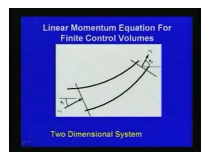
Similar way we can write for two dimension system for a two dimension system if you consider the  $f_x$  the force is in x direction is equal to rate of change of momentum is equal in x direction that is equal to rate of change of mass into change in velocity in x direction rate of change of mass if any mass change takes place. If you put a dash is the rate of change of mass change in velocity in x direction.
