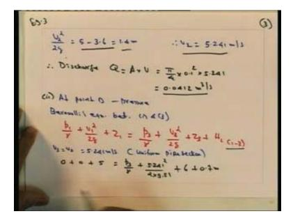
Finally, we get the discharge as 0.0412 meter cube per second. Then, the second part of the question here is we are asked to find the pressure at highest point d to find out the pressure at point d. We will again consider here the figure, we will consider the
