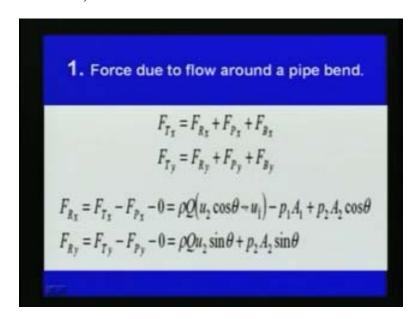
We found the force in x direction y direction we can find out the resultant force that is the thrust required to keep the pipe the that pipe the thrust block should withstand this force. This is one of the simple application of the momentum linear momentum equation. Further we will be discussing some more applications of this linear momentum equations in the next lecture.
