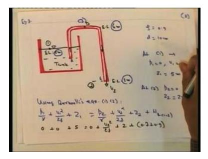
Here we have got a tank and a siphon is used to empty the oil from this tank like this using a siphon and question is the oil surface in the tank is at an elevation of 5 meter and siphon discharges to atmosphere at an elevation of 2 meter. Center line of siphon at its highest d is at an elevation of 6 meter the losses in pipe to higher is 0.7 meter and 0.9 meter from higher point to outlet.
