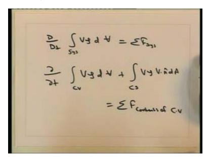
Now with respect to the equation which we derived if you consider here the linear momentum equation for finite control volume, shown here, considers a pipe flow like this.
