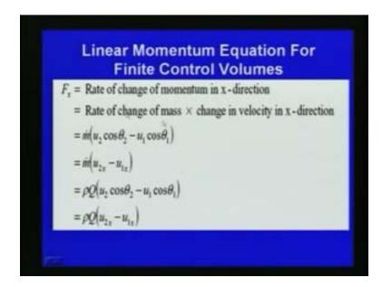
With respect to this figure (Refer Slide Time: 37:12) we can write as  $u_2$  cos theta<sub>2</sub> minus  $u_1$  cos theta<sub>1</sub> if theta<sub>1</sub> is the angle here and theta<sub>2</sub> is the angle here with respect to the x
