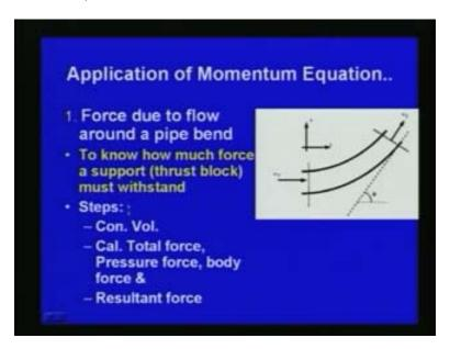
We want to know how much force is required to force should be there to support or the thrust block must withstand is there is a thrust block, here the force the flow is taking place in this bend pipe, we want to find how much is the thrust block how much thrust should be put that.
