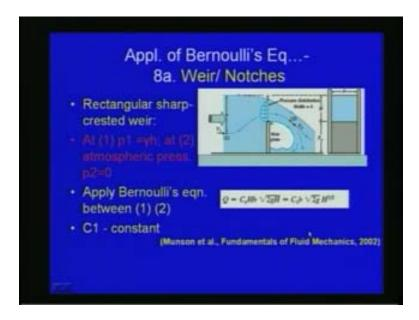
This way here also  $p_1$  equal to  $p_2$  equal to 0 and then by using the Bernoulli's equation and continuity equation we can find the discharge passing through this sluice gate. This is one of the applications as far as open channel flow is concerned and then another application is application for the Bernoulli's equation for weir or notch. So, here we can see that weir is here so we want to find how much is the discharge passing over the weir um or a notch.
