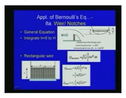
Again, here if you consider a general equation for the weir or notch the general equation you can see is the sharp crested weir and then you consider a small strip of elemental strip through a notch. You can see that this velocity u is equal to square root of 2 g h and discharge through the strip delta Q is equal to area of cross section into velocity V into delta h into square root of 2 g h with respect to this figure here.
