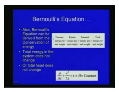
For Bernoulli's equation as you can see in this slide, the Bernoulli's equation can also be derived from conservation of energy. We have seen the energy per unit weight plus the pressure energy plus unit weight plus kinetic energy per unit weight plus potential energy per unit weight is equal to total energy per unit weight of the system. We have already seen that the total energy in the system does not change as per the conservation of energy;
