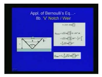
Similarly, if you consider a V notch as shown in this figure, again, this V notch is just a triangular weir, here this b width at this particular location can be found at depth h from the surface of the water in the total depth is H; so b is equal to two times H minus H into tan theta by 2 is the angle of the V notch. Then, Q<sub>theoretical</sub> is equal to 2 into root 2 g tan theta by 2 integral 0 to H minus h into square root of h d H.
