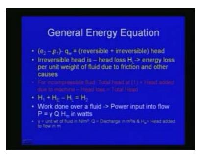
Now,  $e_2$  minus  $e_1$  minus  $q_w$  can be written as reversible plus irreversible head. Irreversible head is can be written as head loss and it is the energy loss per unit weight of fluid due to friction and other causes. For incompressible fluid we can write total head at 1 plus heat added due to machine like pumps or turbine and then minus head loss is equal to total head
