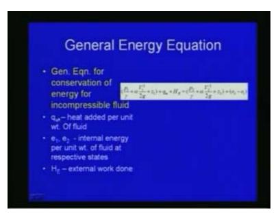
General equation for conservation of energy for incombustible fluid between two sections we can write as p1 by gamma plus alpha V1 square by 2 g plus z1 plus  $q_w$  plus H E is equal to  $P_2$  by gamma plus alpha  $V_2$  square by 2 g plus  $z_2$  plus  $e_2$  minus  $e_1$ , where this  $q_w$  is the heat added per unit weight of fluid so that effects is to be considered.  $e_1$  and  $e_2$  are the internal energies, it is there where the flow is considering and H E is the external work done.
