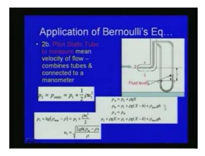
In earlier case what we discussed should have one piezometer and a pitot tube. But instead of this arrangement, we have another type of arrangement to find out the mean velocity of fluid, pitot static tube in this figure. You can see that a pitot static tube is
