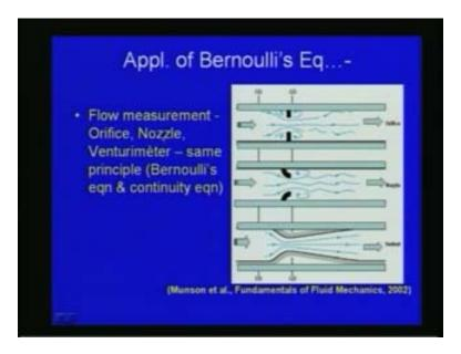
Then nozzles and venturimeter which we have already discussed are some of the equipments used for flow measurements which we utilize the Bernoulli's equations and continuity equation together. So that we can find the flow of velocity over the discharge at particular sections of a pipe line especially the mechanism is used for pipe line. This is one of the applications of the Bernoulli's equation
