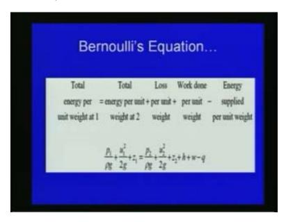
We can utilize this principle in many forms including, considering the total energy of the system including the work done per unit weight or the energy supplied per unit weight as we can see in this slide.
