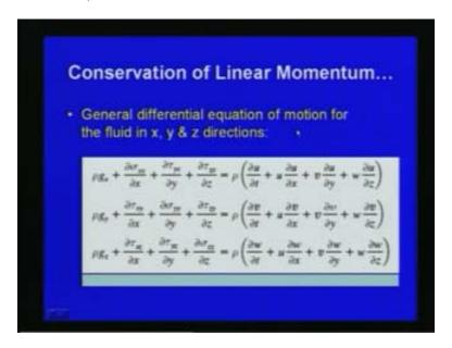
So by using Newton's second law we have equated the forces into the mass into acceleration, the forces are concerned we have seen the body forces and surface forces. By equating by using Newton's second law if you get then we can see that this is in x direction the equation will be rho g x which is the body force in x direction plus due to
