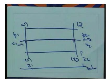
So the Bernoulli's equation, actually when we derive the equation earlier for general one but it is restricted to in viscid flow or non viscous flow, and it is in steady state and the general application is for incompressible flow and flow along a streamline. These are some of the restrictions as far the Bernoulli's equation is concerned. The equation is applicable for in viscid flow since from Euler's equation we have derived and steady state only.
