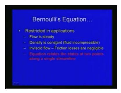
And then of course we also put the assumption that fluid is in viscid, so that friction losses are negligible so this assumption is actually many of the practical problems it will be difficult to apply but certain times, certain places we can approximate the flow is even though, say the viscosity is to be considered. Whenever water is concerned since its viscosity is small or air flow is concerned viscosity is small.
