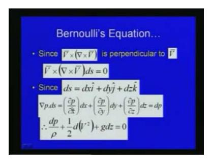
So that finally after using all these approximations the Euler's equation in steady state become d p by rho plus half d V square g d z is equal to zero. So after using all these approximations put forward here in the slides, finally we get this dp by rho plus half d V square plus g d z is equal to zero. So now along the streamline as we discussed here we integrate so that integral d p by rho plus V square by 2 plus g z is equal to constant.
