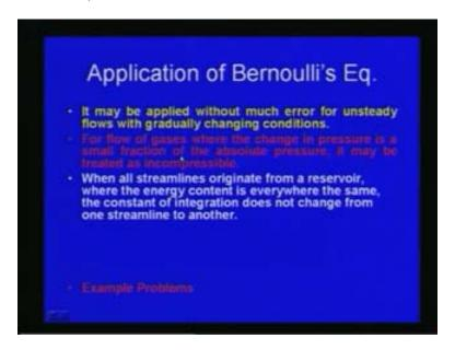
And when all streamlines originate from a reservoir where the energy constant is everywhere, the same constant of integration does not change from one streamline to another. So that this case also we can consider, so this has some of the cases which we can consider the. Bernoulli's equation further equation will be discussing later.
