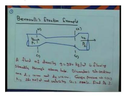
A fluid of density rho is equal to 980 kilogram per meter cubic is flowing steadily through a above tube, here you can see a tube flow a liquid is flowing through this tube and diameter at section 1 is ten centimeter and section 2 it is 12 centimeter and gauge pressure at section 1 is 260 Kilonewton per meter square and velocity here at section 1 is  $u_1$  is equal to five meter per second we want to find  $P_2$ .
