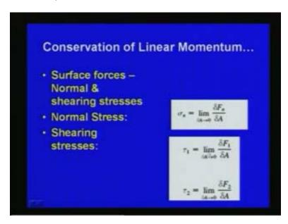
So these are the main surface forces, so we have already seen as far as a fluid element is concerned the important forces are the body forces so that body forces mainly due to acceleration, due to gravity as we have seen here the body forces delta F is equal to delta m into g and then the surfaces forces are concerned there can be normal and shearing stresses.
