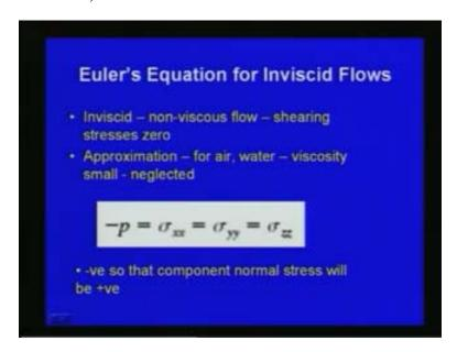
Here the Euler's equation for in viscid flow based upon the general differential equation of motion will be deriving. So Euler's equation is concerned, the equation is valid for in viscid or non viscous flow that means shearing stresses is 0. We have already seen the general equation here.
