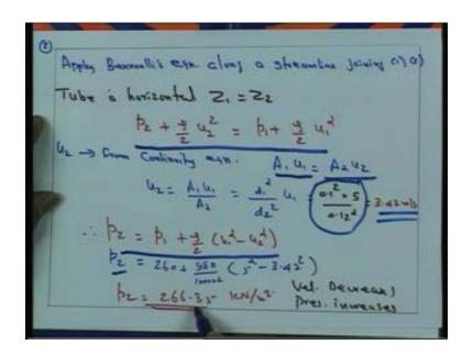
So in this equation all the values  $u_1 u_2$  and  $p_1$  is known. So that we can find  $P_2$  so  $P_2$  is equal to two hundred and sixty six point three five kilo Newton per meter square and we can see that when the velocity is decreased from five meter per second to three point four seven meter per second per pressure is increased from two, two sixty kilo Newton per meter square to two sixty six point three five kilo Newton per meter square.
