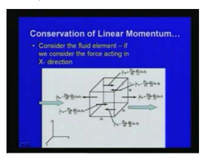
So this is mainly for in viscid flow that means the flow is considered without the viscosity so that is we derived based upon the conservation of linear moment.
