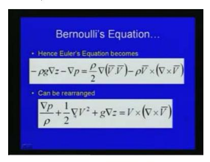
So now we are approximating the Euler's equation into derive the Bernoulli's equation. Now say let us consider a stream line like this as shown in this figure here, so if you take the dot product of each term with a differential length ds along a streamline as shown here this is streamline so that equation will become del p by rho dot d s plus half into del V square d s plus rho del z d s is equal to V cross del cross V d s.
