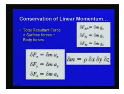
So these are the body force component in x y z direction. Now with respect to the Newton's second law also we have seen earlier with respect to the conservation of linear
