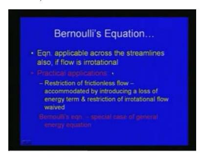
We have already seen, what is rotational flow? What is irrigational flow, in that case irrigational flow, we can say that the Bernoulli's equation is also applicable for across the streamline and some of the practical applications, the restriction frictionless can be considered then it can accommodate by introducing a loss of energy term and restriction of irrigational flow as we have seen here.
