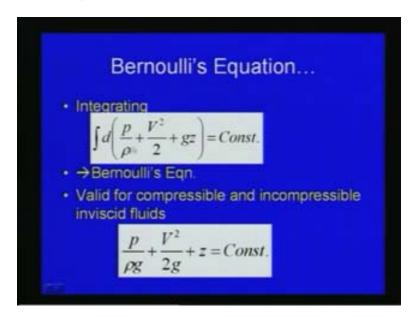
Finally, this gives the Bernoulli's equation, so Bernoulli's equation is actually here are three terms: one is with respect to pressure, other one is the velocity, with respect to velocity square, and the position head gz with respect to z. So this is the integral form this is the general Bernoulli's equation. As we have seen this is valid for incompressible and inviscid fluid.
