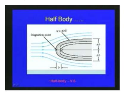
You can see the source and the uniform flow. Due to the effect of the source, the uniform flow streamlines will be deflected both sides like this. Due the source, the streamlines are coming to this point, the source. Finally, we get the half body. It is like a solid surface due to the closed streamline, that is why, it is called a half body.
