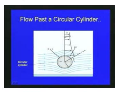
The above figure shows the flow past a circular cylinder. You can see that, this is a combination of doublet and uniform flow. Next, we will define all other properties for a flow past a circular cylinder.
