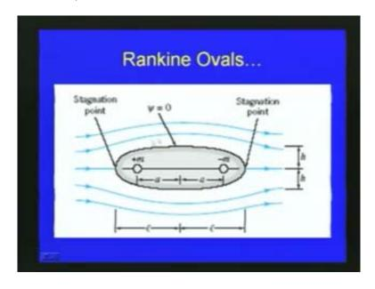
If streamlines are plotted, you can see that, psi is equal to 0; forms a closed boundary as shown in the figure. The stream function is equal to 0. Since body is closed, all of flow emanating from the source, flows into the sink. These bodies having an oval shape is called Rankine ovals.
