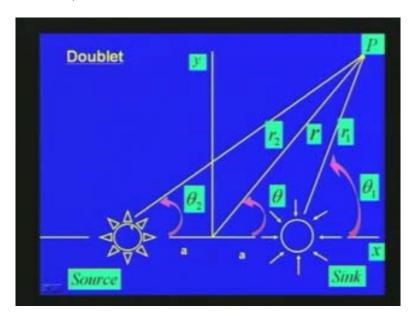
There is a source of strength m and here there is a sink of strength m, and then this is the origin. The source and sink are separated by distance, a on the left hand side and a on right hand side. The r is defined, with respect to point P,  $r_1$  and  $r_2$  is defined, with respect to source and sink; and angle theta one, theta two, and theta is defined. You can see the direction of x-axis and y-axis.
