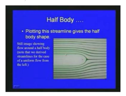
We can plot this streamline with respect to the half body shape. This is the still image showing flow around a half body. So, a half body is obtained, by superposing a source in a uniform flow. We have already defined the velocity potential, the stream function, the radial velocity and the tangential velocity. We have seen the stagnation point and also how all this parameters are derived, with respect to the discussion on this half body.
