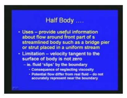
This concept of half body is useful, as it provides useful information about flow around a front part of a streamline body, such as a bridge pier or a strut placed in a uniform stream. The limitation is, velocity tangent to the surface of body is not 0, that is, fluid slips by the boundary. So, the assumption consequence of neglecting the viscosity is that the fluid slips by the boundary and potential flow differs from real fluid. So, do not accurately represent near the boundary.
