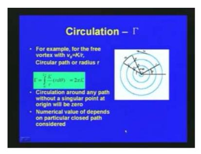
If you consider the circulations here, as you can see this figure, with respect to the velocity v subscript theta and with respect to the radius r, here theta is mentioned. For example, for the free vortex with v subscript theta is equal to K by r, circular path of radius r can be described as, gamma is equal to, integral 0 to 2 phi K by r into rd theta is equal to 2 phi K.
