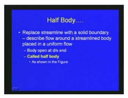
From this discussion, we can say that, if you replace the streamline with a solid boundary, this describes flow around a streamlined body, placed in a uniform flow. The body open at the downstream end is called the half body. This is shown in the figure below.
