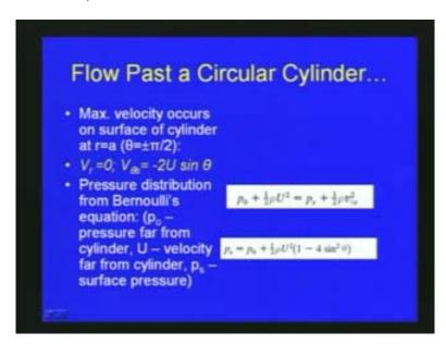
The maximum velocity occurs on a surface of cylinder, at r is equal to a; where theta is equal to plus or minus phi by 2, as shown the figure; the radial velocity  $v_r$  is equal to 0 and tangential velocity on the surface of the cylinder, v subscript theta s, is equal to, minus 2U sine theta. U is the uniform flow velocity.
