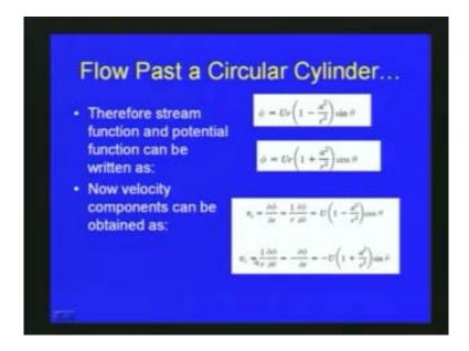
Therefore, the stream function and potential function for flow past a circular cylinder can be written as: psi is equal to Ur into 1 minus a square by r square sine theta and the velocity potential phi is equal to Ur into 1 plus a square by r square cos theta.
