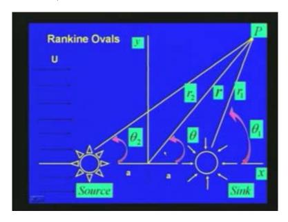
In this figure, you can see that, there is a source here and there is a sink here. There is uniform flow of velocity U. A Rankine oval is obtained by superimposition of this source and sink of the equal strength at distance a. Finally, the shape of the Rankine ovals is obtained.
