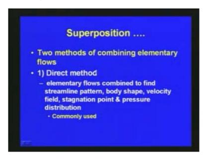
In the direct method, the elementary flows are combined to find the streamline pattern, the body shape, the velocity field, stagnation point and pressure distribution. We are directly superposing the various parameters like stream function and potential function. This direct method is most commonly used. The second method of superposition is called inverse method.
