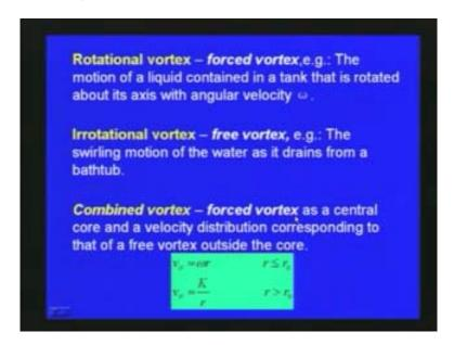
So the circulation is an important parameter which we use as for as rotational vortex or irrotational vortex is concerned. We have also defined the tangential velocity for the vortex as v subscript theta is equal to omega r or v subscript theta is equal to K by v, where v is greater than v0, as described earlier.
