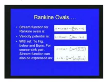
The stream function for Rankine oval can be defined; psi is equal to Ur sine theta, which corresponds to the uniform flow, minus m by 2 phi theta<sub>1</sub> minus theta<sub>2</sub>. Velocity potential is defined as; psi is equal to Ur cos theta minus m by 2 phi natural log r 1 minus natural log r 2.
