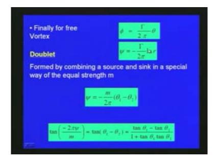
For a free vortex flow with respect to circulation gamma, the potential velocity phi is equal to, gamma divided by 2 phi theta, and psi the stream function, is equal to minus gamma by 2 phi into natural log r; where gamma is the circulation and r is defined and theta defined. We have already seen earlier the general definition of phi and psi, where phi is equal to K theta and psi is equal to minus K natural log with respect to the circulation gamma, we can define the free vortex phi and psi.
