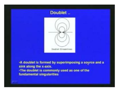
As respect to the previous slide as the source and sink approaches to the origin, you can see the doublet streamlines this are plotted like this. So finally, we can say that doublet is formed, by superimposing the source and a sink along the x-axis. The doublet is commonly used as one of the fundamental singularities. This is the definition of the doublet and the various parameters are discussed.
