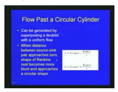
Rankine oval is obtained by, superimposition of a source and sink of equal strength, at distance a, within a uniform flow. It is another way of combination of simple elementary flows to get a complex flow system. The third case, we will discuss the flow past a circular cylinder.
