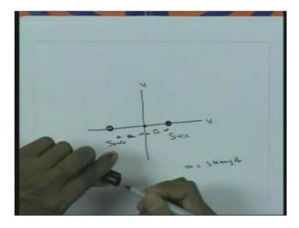
Now, we will say that a doublet is formed by letting the source and sink approach one another. As shown in the figure, if this is the origin, this is y and this is x. There is a sink and here there is a source, initially there is a distance a here on both sides. So when this a tends to 0, letting source and sink approach one another, so that a tends to 0, m is the increasing strength of source and sink, and m tends to infinity, then we say that a doublet
