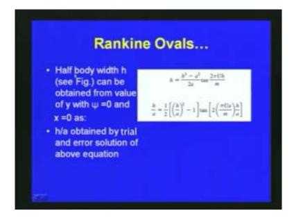
The width of half body can be obtained from the value of y with psi is equal to 0. We can get width of the half body h from the definition of the stream function, when x is equal to 0. So, h is equal to h square minus a square by 2 a tan 2 phi Uh by m, from the previous definitions. We can obtain h by a ratio as, h by a, is equal to half of h by a whole square minus 1 tan of 2 phi Ua by m h by a.
