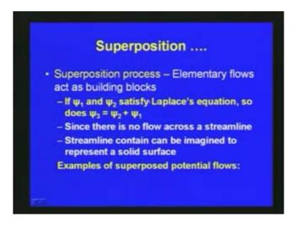
For example, in Laplace's equation, if psi<sub>1</sub> and psi<sub>2</sub>, satisfy the Laplace's equation, that means, if we add this two stream function, psi<sub>1</sub> and psi<sub>2</sub>, so that you will get another stream functions psi<sub>3</sub>. This is the basic principle of this superposition. Since, there is no flow across a streamline and streamlines contain can be imagined to represent a solid surface.
