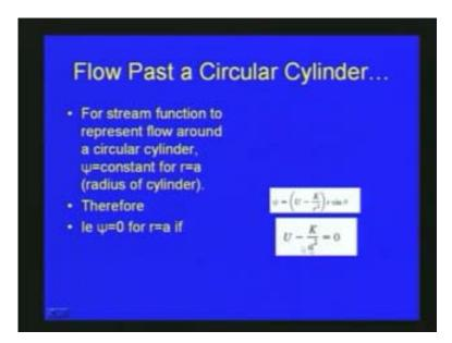
From the figure, you can see, on the surface of the circular cylinder, the stream function can be defined as psi is equal to 0, for r is equal to a; we can define U minus K by a square, is equal to 0.
