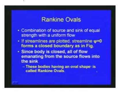
Now, we will see another concept called Rankine ovals. This is also by superposition of two types of elementary potential flows. The Rankine ovals are obtained by combination of a source and sink of equal strength, with a uniform flow. The half body, we obtained by superimposition of a source within a uniform flow, but now we will get the Rankine ovals by superimposing or by combination of a source and sink of equal strength, with a uniform flow.
