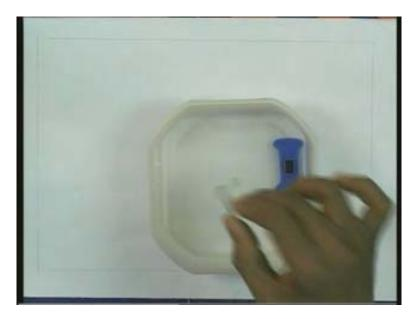
So but you can see in this slide if the liquid is wetting type we can see that there will be a small rise like this so that is called capillary rise so this the liquid is you can see that both surface it is wetting for that is why due to the cohesion it is a rising is taking place and that is what is called capillary rise.
