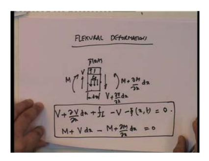
So, we will look at flexural deformation and if I take any d x what do I have, I have M M plus del M by del x d x then I have V then I have V plus del V by del x d x. Then I have load P bar x of t and on top of that, since this is moving up in this direction, I also have f I. So, if I were to look at the two equations, what do I get, I get two equations, there is a force equation in this direction. So, if you look at the force equation, what I get is, V plus
