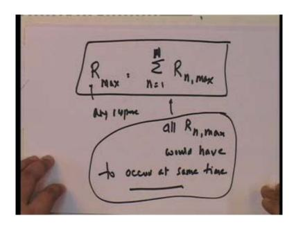
Now, one of the things that you could say is that well. So, what could I find out for example, R max is equal to summation n going from 1 to n R n when, R is any response could I say that, this is the problem with this is that although this is valid for any instant of time, for this to be valid what would happen, all R n max would have to occur at same time right, so this mode superposition all though it is valid when you are doing time history because at any instant of time you can add up.
