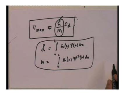
So, if you look at it the peak displacement is equal to L upon m into s d. So, that is becomes my solution and then of course, you know we can find out what do you want to find out, we want to find out the shear force. The shear force etcetera, we can always find out, but in a sense the point that I am trying to make is that there is a term, which is been brought in where L is equal to 0 to L m bar x psi x d x and m is 0 to L m bar x psi square x d x.
