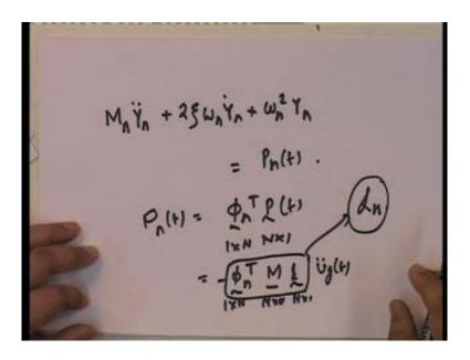
So, the modal amplitude equation looks like, M n y and double dot and here I can incorporate my damping, y n double dot plus omega n square y n is equal to p n of t well what is p n. P n if you look at it is nothing but p n of t is equal to phi n transpose p of t this is 1 by N, this is N by 1, this is 1 by 1 scalar. Now, here in this particular case p n of t a p of t is equal to, so I am going to say phi n transpose I am going to put minus m into 1 into v g of t.
