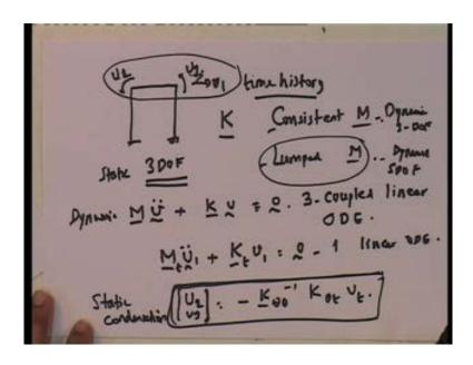
And if I use the lumped mass, I showed that all you needed to do was solve, which is one linear ODE and you needed to solve, then once you solved for v 1, v 2 and v 3 you could get from minus k theta theta inverse k theta t v t. So, in other words we still it is not as, if this is still 3 degree of freedom structure, nobody can take away from the fact, that this is a 3 degree of freedom structure.
