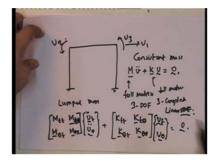
If you look at the structure level, let us look at this structure v 1 and v 2, v 3, so this is the structure that we have been looking at. Under the consistent mass formulation, what do we have, we have m bar v double dot plus k v and I am going to put 0 now, because I am not looking at loading at all at this particular situation. So, this and here, full matrix, this is the consistent mass formulation, this is the full matrix and so we have to solve a three degree of freedom.
