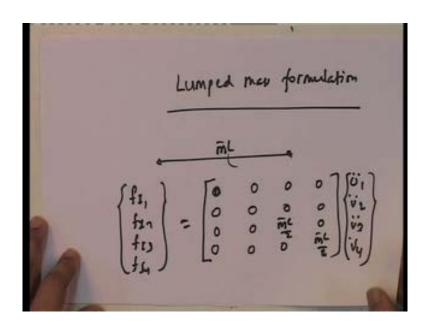
Since they do not have any rotatory inertia, what is the mass matrix look like, in a lumped mass formulation what we have is that, m bar L is a total and so my inertia f i 1 f i 2 at the member level, f i 3 i 4 is equal to 00000000000000000 m bar L by 200 m bar L by 2. Note that, in the lumped mass formulation, since I put point masses here and I have taken the kind of displacement for v 3 as this and for v 4 as this, I get m bar L and they do not contribute any force over here.
