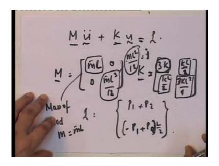
So, finally, what does it look like well, m into u double dot plus K into u is equal to p and note this time, that since you see, you see this equation this equation has u x and u theta and this equation has u theta and u x. So, they are not uncoupled, since they are not uncoupled, its actually 2 simultaneous differential equations and that is why you have this if m or k or both are not diagonal matrices, then automatically the system becomes coupled.
