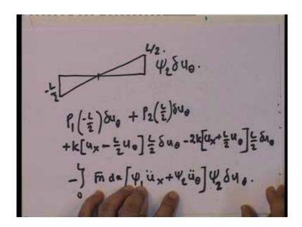
So, we got the first equation and now what we need to do is we need to define another virtual displacement pattern, a which is not is not included in the other pattern. So, if we do this the obvious 1 to do is a virtual displacement pattern, which is like this and where you know this is minus L by 2, this is L by 2, so if we get this pattern then what is the virtual displacement virtual work equation look like let start, the first one is the p 1 here.
