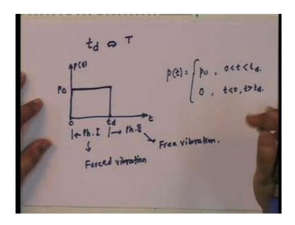
Short duration essentially implies that if I call t d, as the duration of the pulse, this is of the same order of magnitude as the time period of the structure, when I say same order of magnitude I essentially mean that they are similar to each other. It is not as if t d is equal to it just means that t d could be t by 2, could be t by 4, could be 2 t, but not more than 2 t for sure.
