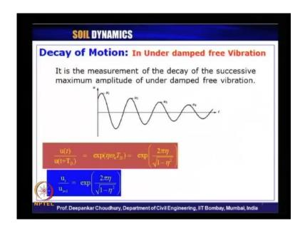
So, decay of motion, it is the measurement of the decay of the successive maximum amplitude of under damped free vibration. So, what does it mean? If u 1 is the maximum amplitude here, and u 2 is the maximum amplitude in the second cycle, u 3 is the maximum amplitude at the third cycle, u 4 is the maximum amplitude at the fourth cycle then the decay or the logarithmic decrement.
