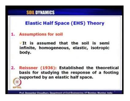
So, this is the third or the last method. We have discussed that, there are basically three methods to analyze or design a machine foundation. One is Tschebotari-off's reduced natural frequency method, which we have studied thoroughly and also we have solved the problems; we have practiced it. Then we have seen mass spring dashpot model; that also we have studied thoroughly and we have seen how its practice can be made. Now,
