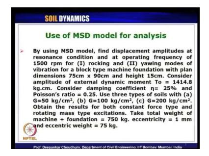
A quick recap of what we had studied in the previous lecture; we have solved the problem using mass spring dashpot model for computing the displacement amplitude at both resonance condition as well as at operating frequency condition for rocking and yawing mode of vibration. Let us now move to yawing mode of vibration. Yawing is nothing but torsional mode of vibration.
