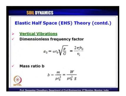
So, that is how for vertical mode of vibration, you can see in this slide, the dimensionless frequency factor is calculated like this. So, if you change from omega to f as you know in the case of hertz if you use the unit of hertz, it will be 2 pi f naught – nothing but omega r naught by v s – shear wave velocity. And mass ratio b is m by rho r naught cube. If you use the weight, then weight by gamma r naught cube you can use.
