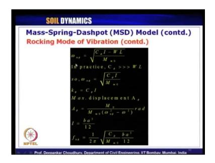
Now, this natural frequency omega m phi that is calculated as root over k phi by m m naught. Now, k phi is nothing but this 1. So, in practice, this C phi is much more than W l. So, we can consider this equals to root over C phi i by m m naught and maximum displacement a phi will be this m naught. That is externally applied moment amplitude divided by m m naught, that is mass moment of inertia of the system about axis o times omega n phi square minus omega square.
