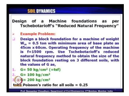
A quick recap of what we had studied in the previous lecture, we have solved a model example problem for design of block type machine foundation using Tschebotarioffs reduced natural frequency method. The problem statement was given to us with the size of the base plate, then weight of the machine, operating frequency of the machine and it was asked for three different types of soil. How we can design the machine foundation?
