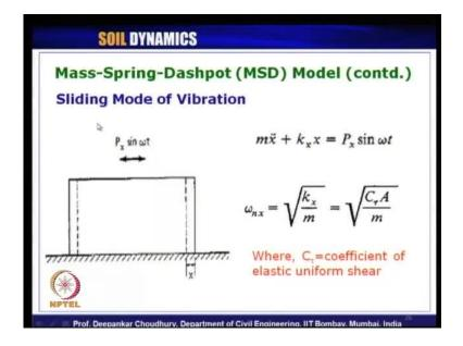
That is sliding mode of vibration, now in the case of sliding mode of vibration this is applied dynamic load and sliding displacement is x. So, our equation of our motion is for
