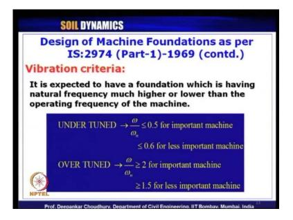
In case of second criteria that is vibration criteria, it says that any machines foundations can be designed either as over tuned or under tuned. In case of under tuned to satisfy the no resonance criteria, the operating frequency and the natural frequency of machine plus foundation system their ratio has to be maintained far away from 1, because they should not be close to each other.
