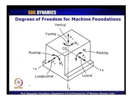
Also we have seen that what are the various degrees of freedom for machine foundations, that is possible deduction of movements like three linear and three rotational deductions of movements or vibration. We name them as this one have vertical vibrations, this one as lateral vibration and this one longitudinal vibrations. These two were also called as sliding mode of vibration or horizontal mode of vibration in x and y direction
