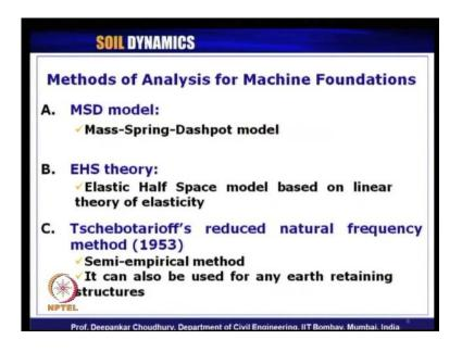
Various methods of analysis are there for machine foundation design, first one is m s d model that is mass spring dashpot model. Second one is e h s theory that is elastic half space theory, based on linear theory of elasticity. Third one is Semi empirical method which is known as Tschebotarioff's reduced natural frequency method.
