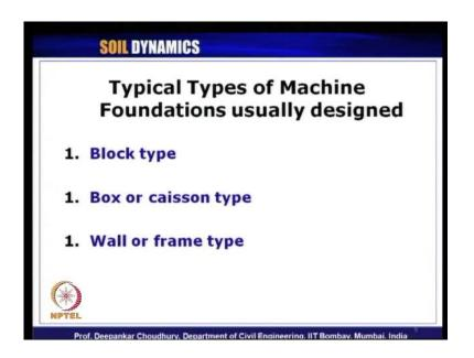
Typical types of machine foundations usually designed are block type, box or caisson type and wall or frame type.
