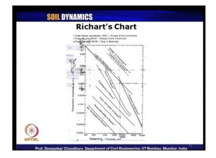
We have seen what is Richart's chart, that is for vertical mode of vibration, how we can find out whether what type of disturbance it is causing. Whether not noticeable to persons to severe to the persons and we should not cross this boundary or limit for design of machine foundation for the design. Similarly, for horizontal mode of vibration also we have seen that type of qualitative chart which we need to satisfy.
