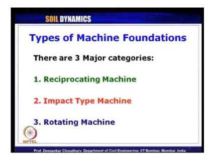
In machine foundations in the previous lecture a quick recap of what we had learnt, there are three major categories of machines, reciprocating machine, impact type machine and rotating type machine.
