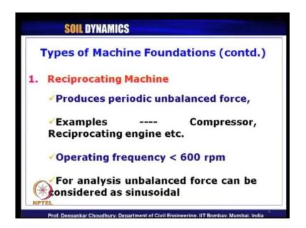
What are their special characteristics that also we have seen, like reciprocating machine produces mostly periodic unbalanced force. Examples of reciprocating type of machines are compressor, reciprocating engine, etcetera, their operating frequency ranges are generally less than 600 r p m. For their analysis we consider the unbalanced force as equivalent to a sinusoidal, because it is a periodic unbalanced force.
