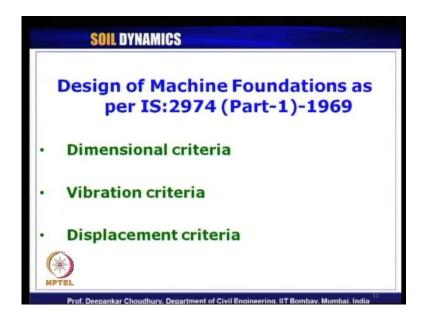
As per Indian design standard code of i s 2974 part 1, the three basic criteria has to be satisfied for the design of machine foundations, dimensional criteria, then vibration criteria and the displacement criteria.
