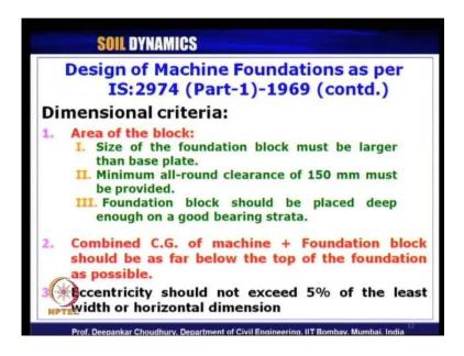
In case of dimensional criteria, we have seen how to select first the area of the block foundation. It says that the size of the block must be bigger than the base plate size on which the machine is placed and a guide line is provided that minimum all around clearance of 150 millimeter has to be provided. The foundation block should be placed deep enough on good bearing strata.
