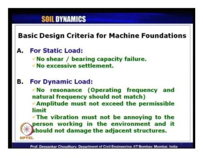
Basic design criteria for machine foundations we have seen, first of all that foundation must be safe against the static load. So, we need to check against that no shear or bearing
