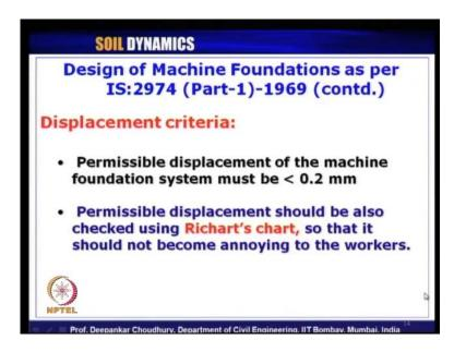
In the third criteria as per our I S code, it is says displacement criteria in that case the permissible displacement amplitude, dynamic amplitude of displacement should be always less than 0.2 millimeter. Another check is that qualitative check what we told you earlier, it has to be checked using the Richart's chart. So, that that displacement is not creating any problem to the people who are staying in the surrounding vicinity or working in the surrounding vicinity.
