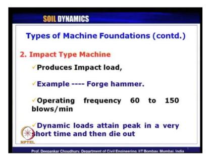
For impact type of machine it produces impact load as the name suggest. Example of such machine is forge hammer and operating frequency is generally between 60 to 150
