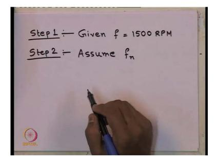
So, let us see step wise, in step one the given value of operating frequency is 1500 r p m, it is given to us. So, the step two says assume f n that is natural frequency of the machine plus foundations system.
