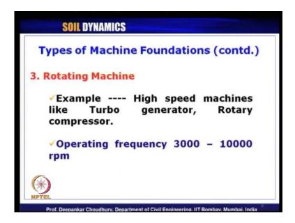
In case of rotating type of machine examples are high speed machines like turbo generators, rotary compressors, etcetera. And operating frequency ranges between about 3000 to 10000 of r p m.
