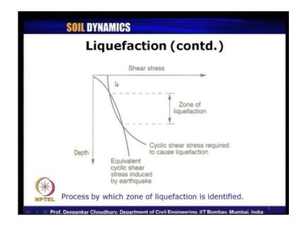
So, this is the basic principle of what we understand by liquefaction. This curve shows the development of equivalent cyclic shear stress induced, because of a particular earthquake and this curve shows cyclic shear stress, which is required to cause liquefaction. So, this is the capacity of the soil. So, if it is less than whatever is produced cyclic shear stress; obviously, the liquefaction is going to happen. So, that is why in this zone we found this is the zone of liquefaction.
