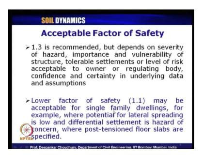
And what are the acceptable factors of safety for design against liquefaction; 1.3 factor of safety is recommended for important structure, whereas lower factor of safety of 1.1 can be used for less important or small buildings like that.
