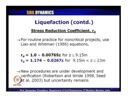
So, stress reduction coefficient r d for routine practice for noncritical projects, Liao and Whitman in 1986; they had proposed equations to compute the values of r d. They have proposed these two expressions that is r d equals to 1 minus this 0.00765 z where z has to be used in meter, z is a depth below ground surface in meter unit because as u know semi-empirical expressions are always unit biased. So, you should remember it is in meter unit.
