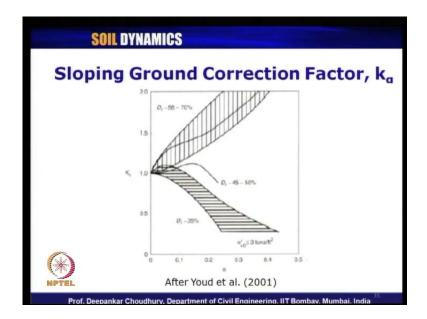
So, the same curve has been reproduced by Youd et al. in 2001 and obviously if you do not have any sloping ground; if it is horizontal ground, alpha will be 0, you do not have to incorporate any value of k alpha; it will be one always as expected.
