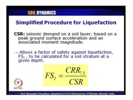
So, two terms have been defined; CRR cyclic resistance ratio and CSR cyclic stress ratio. The factor of safety against liquefaction is defined as CRR 7.5; 7.5 denote the moment magnitude of earthquake of 7.5. CRR is calculated at that magnitude of earthquake by the CSR at a particular depth.
