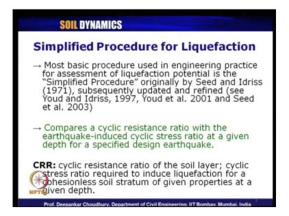
A quick recap of what we had studied in the previous lecture; we had learnt the simplified procedure for estimation of liquefaction potential as proposed by Youd et al. 2001. Initially the simplified procedure was proposed by Seed and Idriss in 1971 which has been subsequently updated and modified and Youd et al. 2001; this is the one of the latest methodology used worldwide for computation of liquefaction potential.
