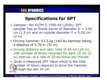
So, specifications for SPT as per ASTM D standard, standard number of this, SPT sampler has an inside barrel diameter of about 3.81 centimeter which is about one and a half inch and outside diameter of about 5.08 centimeter which is about two inch. We know why the sampler dimension also is standardized in terms of inside and outside diameter, why? Because to keep the area ratio of the sampler as minimum, so that the disturbances coming to the soil sample collected in the sampler are minimum.
