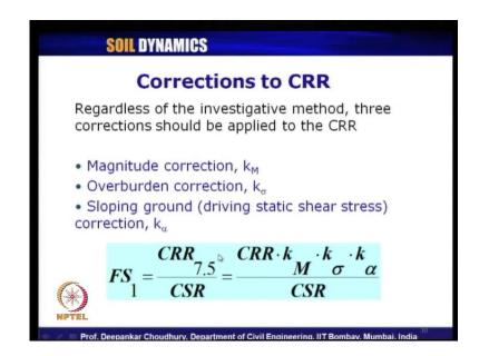
So, corrections to CRR what we have discussed just now; regardless of the investigative method, three corrections must be applied to CRR. These are the magnitude correction; it is denoted by K suffix M, M means magnitude. Overburden correction, K suffix sigma; sigma denotes the overburden stress. And sloping ground, this is due to the driving static shear stress correction which is given by K alpha; alpha is the angle of sloping ground with respect to horizontal.
