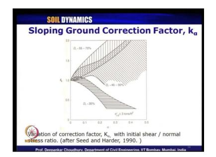
Now coming to the third correction factor that is sloping ground correction factor K alpha. For K alpha, it was initially the correction factor was proposed by Seed and Harder in 1990. So, this itself is transferred to the methodology given by Youd et al.
